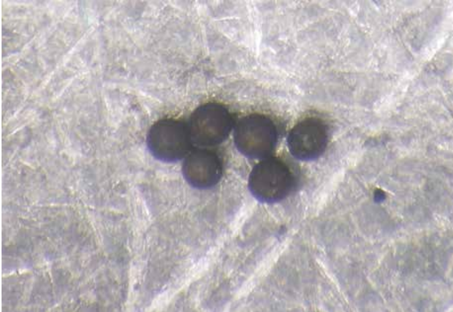
Figure 4. Closeup of one set of UN kernels after irradiation.
