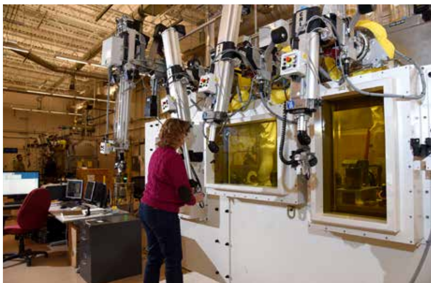
Figure 1. The EPMA instrument scientist (Ms. Karen E. Wright) performing a sample loading operation on an irradiated sample.
