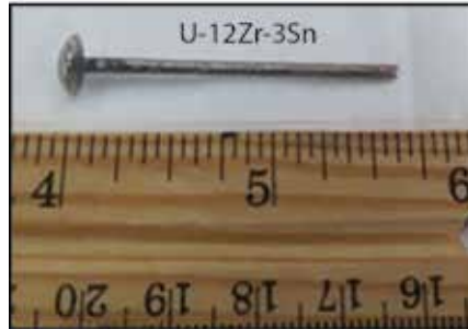
Figure 1. Mockup hardware for the FAST irradiation test to be used in the ATR outboard A and Small I positions.
