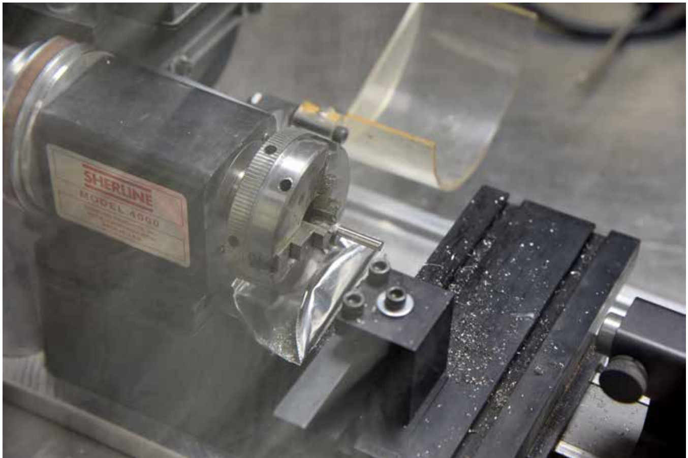
Figure 1. Modified hobby lathe with fuel slug in the chuck to be machined.
