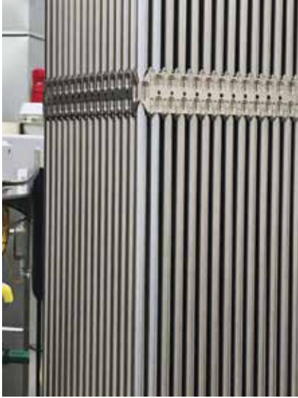
Figure 2. ANO EATF LTAs with two chromium-coated rods in corner of outer row.
