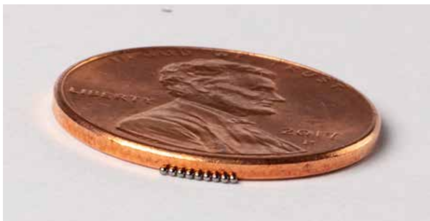
Figure 1. Uranium mononitride (UN) kernels tested in the initial MiniFuel irradiation experiment (photography credit to Carlos Jones/Oak Ridge National Laboratory (ORNL), U.S. Department of Energy (DOE)).
