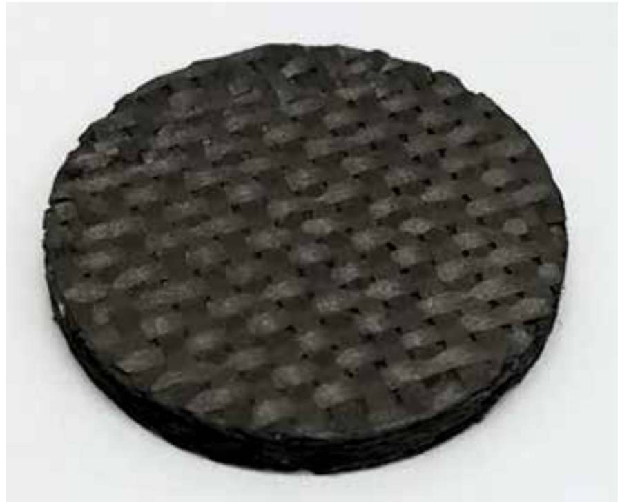
Figure 2. 25mm diameter SiC/SiC composite fabricated with new lab scale CVI system.
