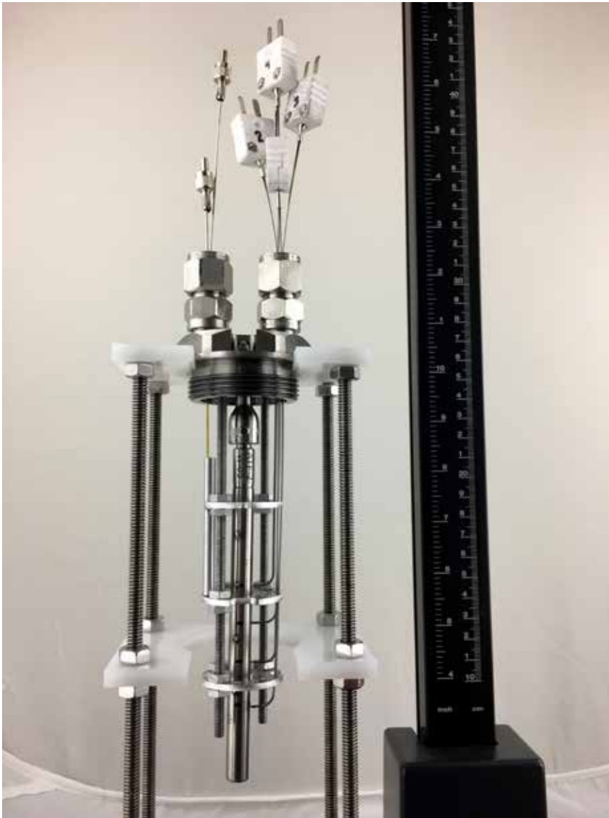
Figure 1. Photograph of the ATF-SETH capsule with two pyrometers located on the left side of the rodlet.
