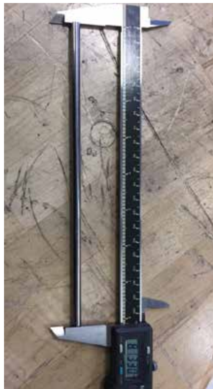
Figure 3. Thin-wall 14YWT tube after pilgering – length 8.13 Inches.
