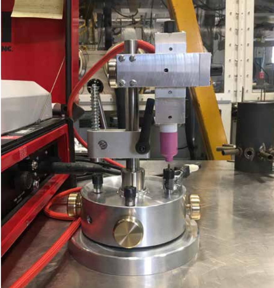
Figure 3. Welding and loading fixture to be used for FAST rodlet fabrication, shown before glovebox installation.
