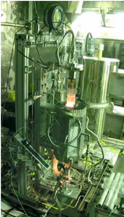
Figure 3. The Severe Accident Test Station pictured during HBR#1 testing. The test station includes the integral LOCA testing module (foreground furnace) and the BDBA high-temperature furnace test apparatus (behind).
