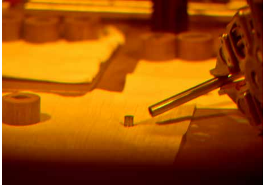
Figure 2. Retrieval of the H-cups in HFEF.
