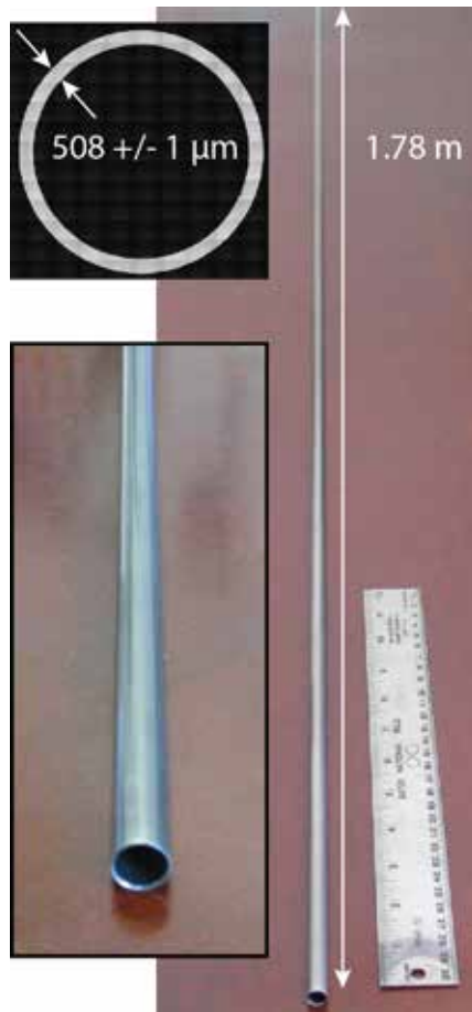
Figure 3. Optical images of the OFRAC thin wall tube and cross-section of the tube (inset)
