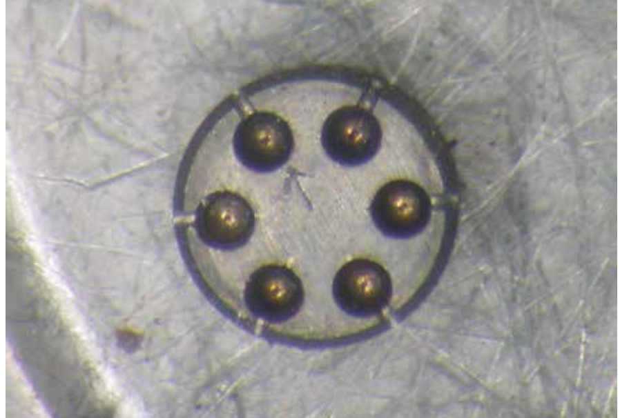
Figure 3. Hot cell extraction of one set of UN kernels contained inside a molybdenum cup.
