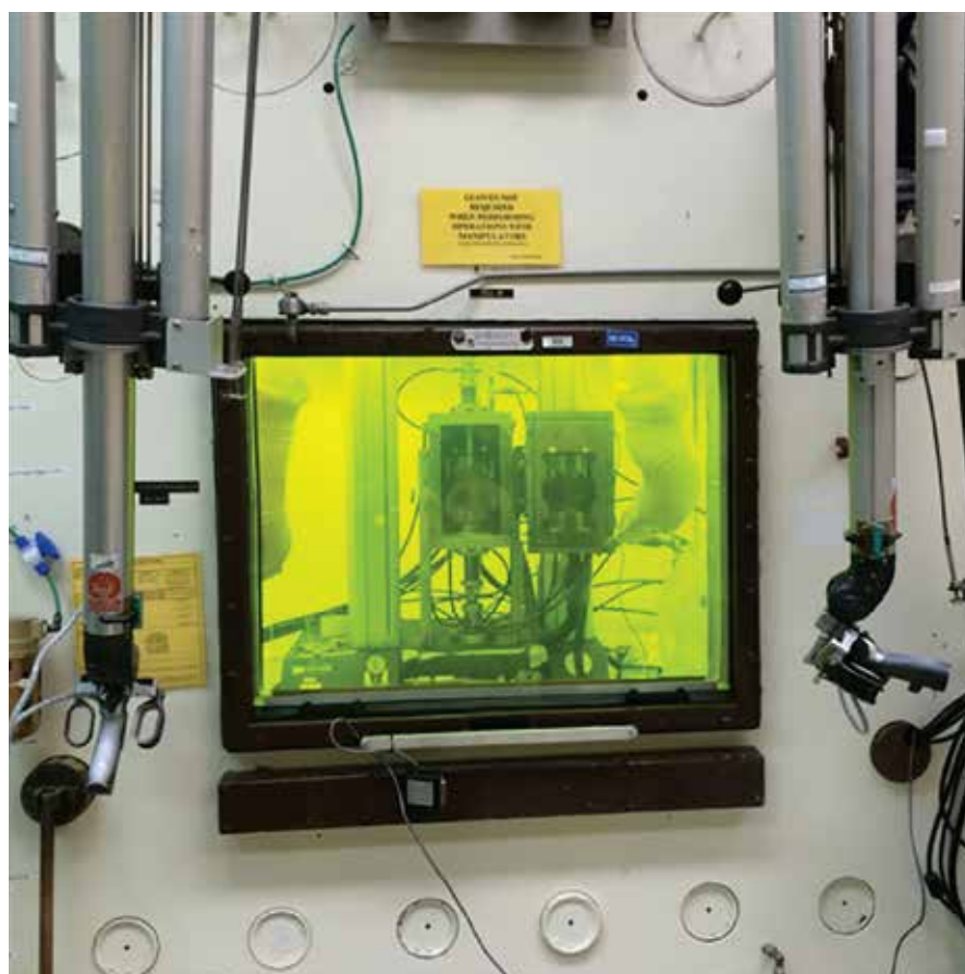
Figure 1. Image of hot cell at Los Alamos National Laboratory (LANL) in CMR Wing 9 where mechanical testing occurred.
