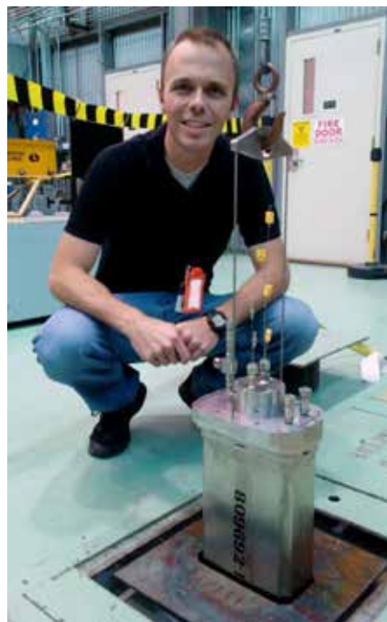
Figure 2. First SETH capsule installed in the irradiation vehicle suspended over a storage hole at TREAT.
