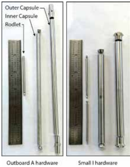
Figure 1. Mockup hardware for the FAST irradiation test to be used in the ATR outboard A and Small I positions.
