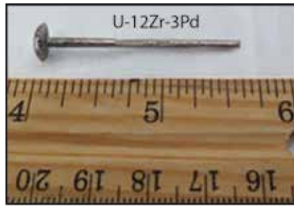
Figure 2. Prototypic FAST fuel slugs casting using the pressure differential assisted gravity casting technique.
