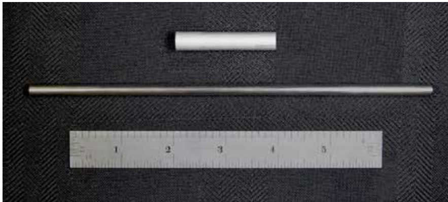
Figure 2. 14YWT starting thick-wall tube and thin-wall tube after pilgering.
