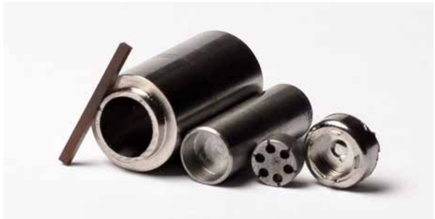
Figure 2. MiniFuel capsule components (photography credit to Carlos Jones/ORNL, DOE).
