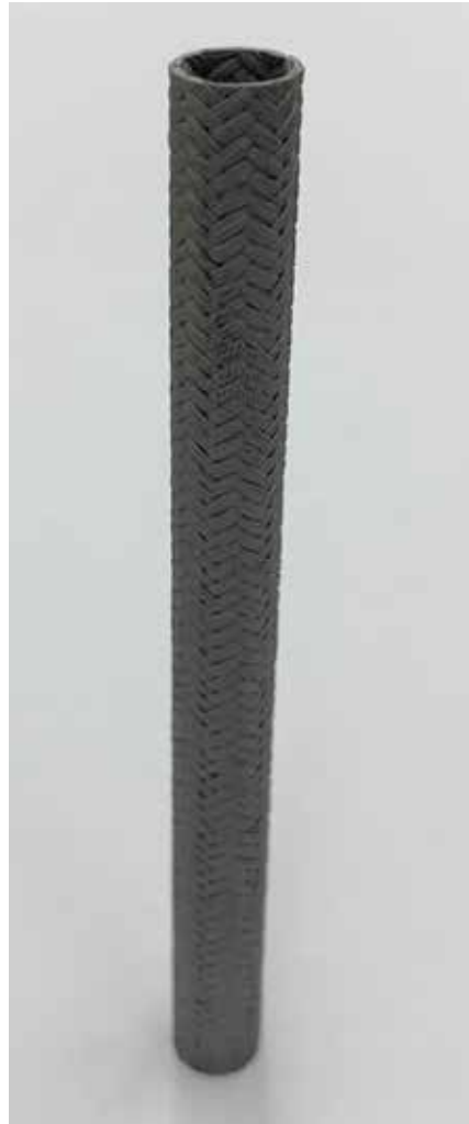
Figure 1. Image showing SiC fiber-reinforced SiC matrix composite tube coated with CrN. The tube length is 110 mm.
