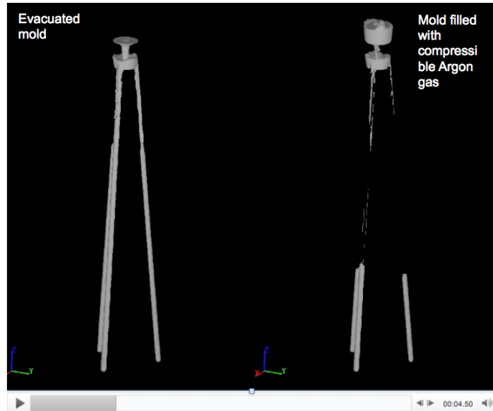
Figure 42. A snapshot of casting with and without argon at 4.5 seconds.
