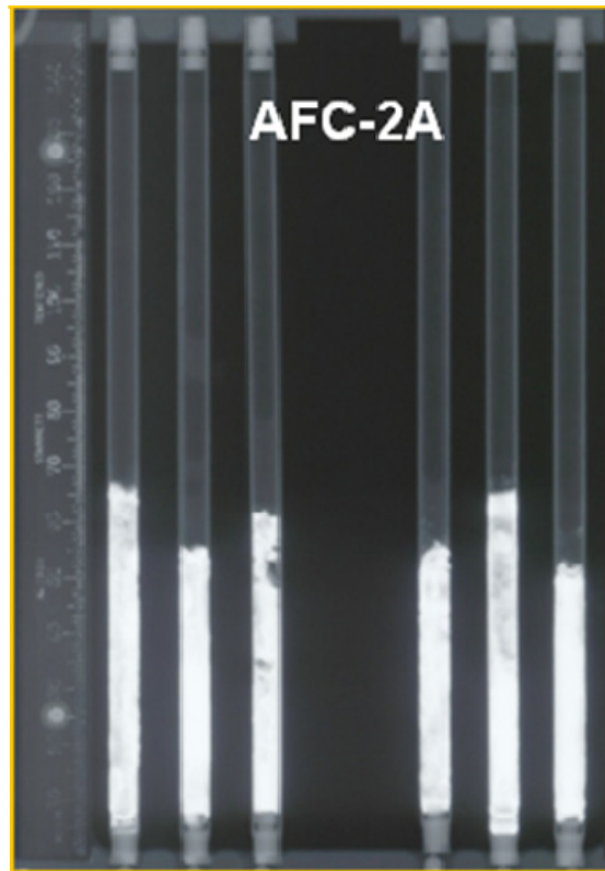
Figure 74. Neutron radiography of AFC-2A rodlets (left to right: rodlet 2, rodlet 1, rodlet 3, rodlet 5, rodlet 6, rodlet 4).
