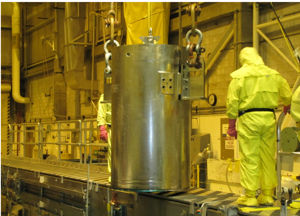
Figure 67. GE2000 cask being inserted into the ATR canal to insert the AFC experiment capsules for shipment to the Materials and Fuels Complex (MFC) for PIE.
