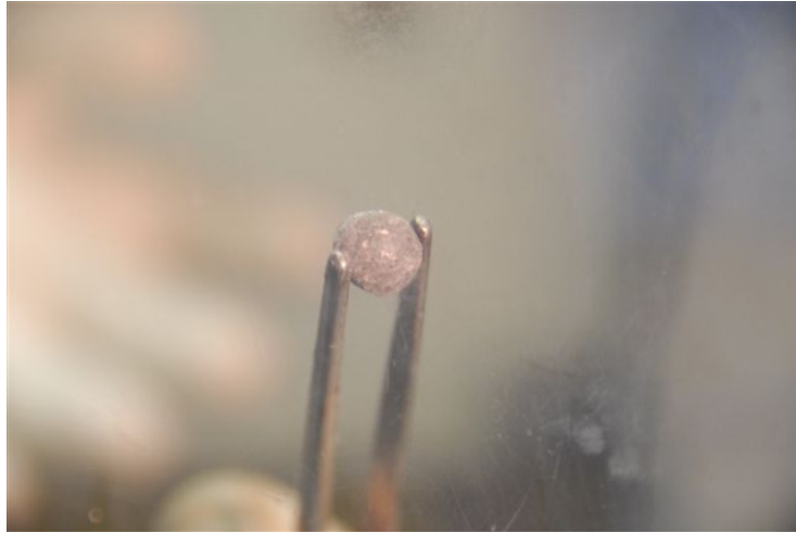
Figure 4. First Np “nugget” formed by direct oxide reduction (DOR) of NpO 2 in stirred molten salt bath.
