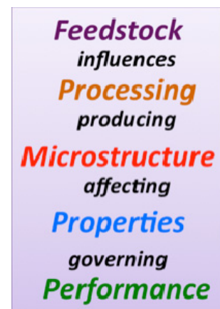
Figure 23. Illustration of materials relationships between starting powder and subsequent fuel performance.
