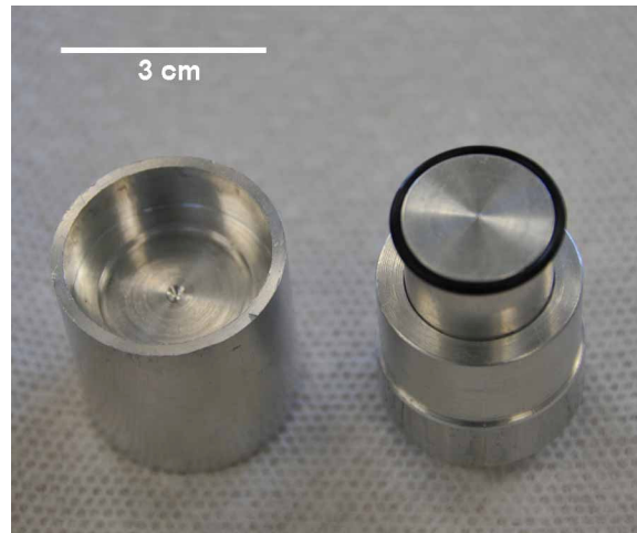
Figure 15. Tool for positioning O-ring on inner dish. Bottom part is on left; piston with O-ring is on right; sleeve is around piston.
