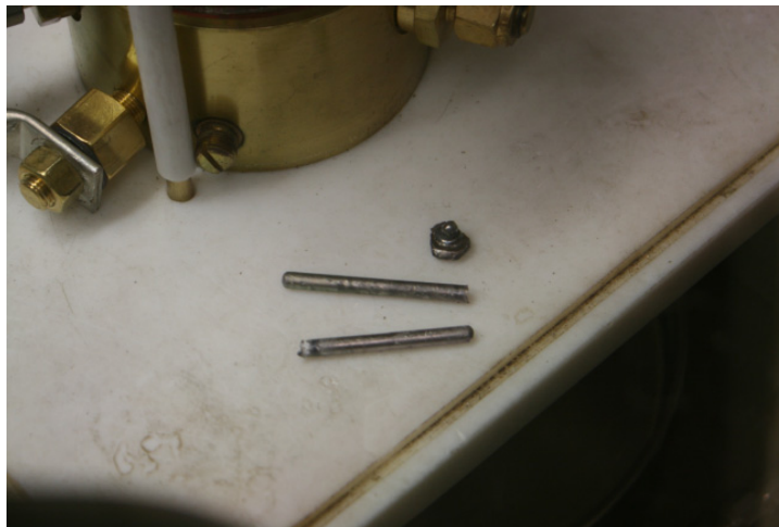
Figure 18. U-Pd-La-Ce-Pr-Nd-Zr alloys cast for characterization.
