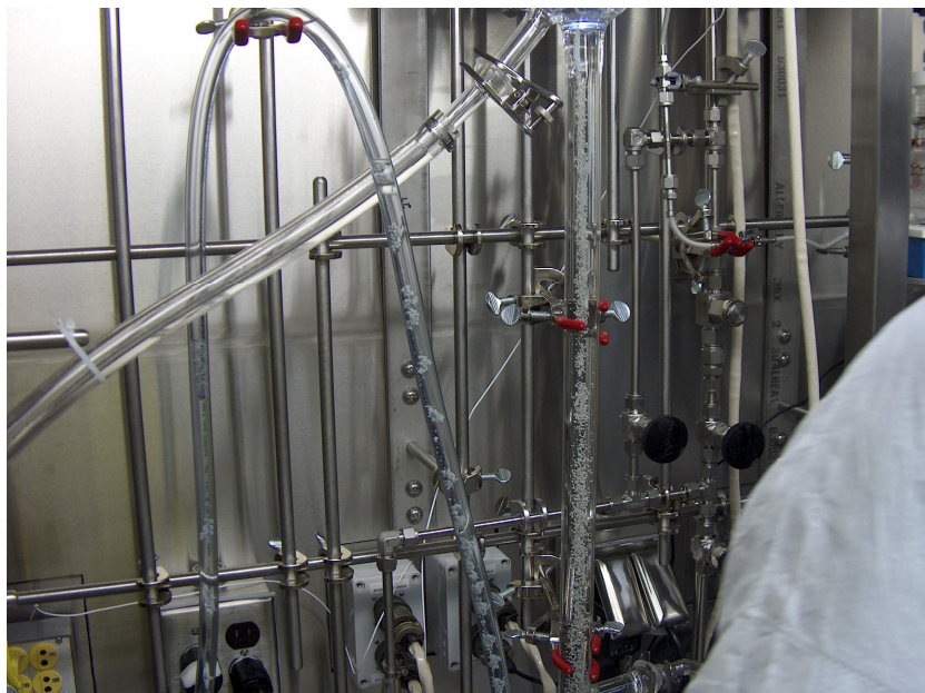
Figure 44. Photograph of the Zr-Y gel spheres containing SiC particles in the gelation column and associated tubing.
