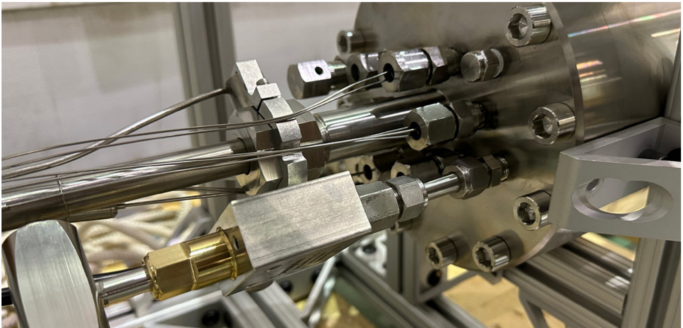
Transient Water Irradiation System in TREAT (TWIST) experiment for LOCA testing.
