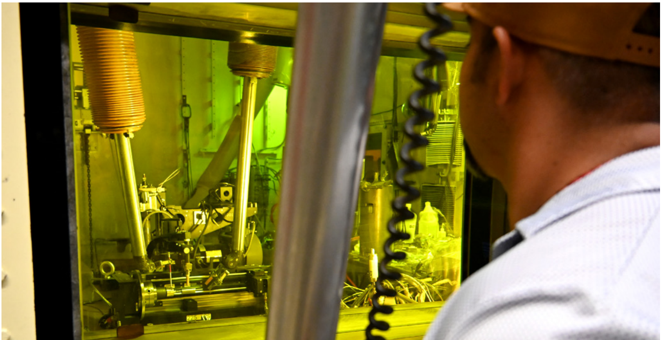
Preparing to perform welds on the High-burnup Experiments in Reactivity Initiated Accidents (HERA-HBU-1) rod.
