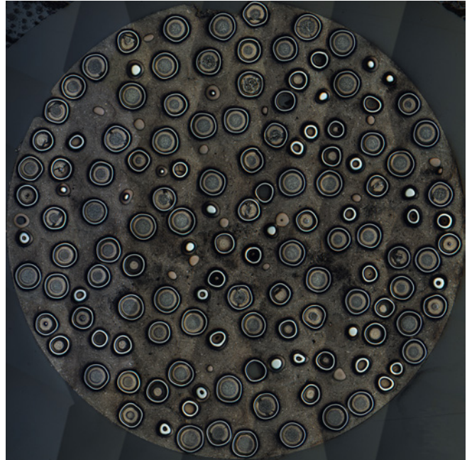
Cross-section of a 1/2-inch-diameter TRISO fuel compact containing poppy-seed-sized fuel particles.
