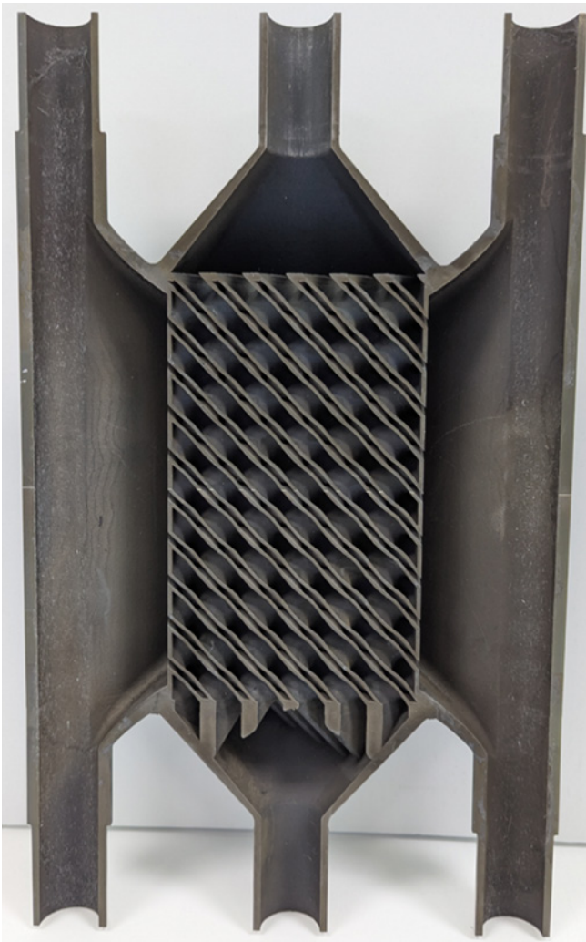
Sectioned view of additively manufactured heat exchanger to test heat transfer properties of advanced nuclear fuel lattice design.
