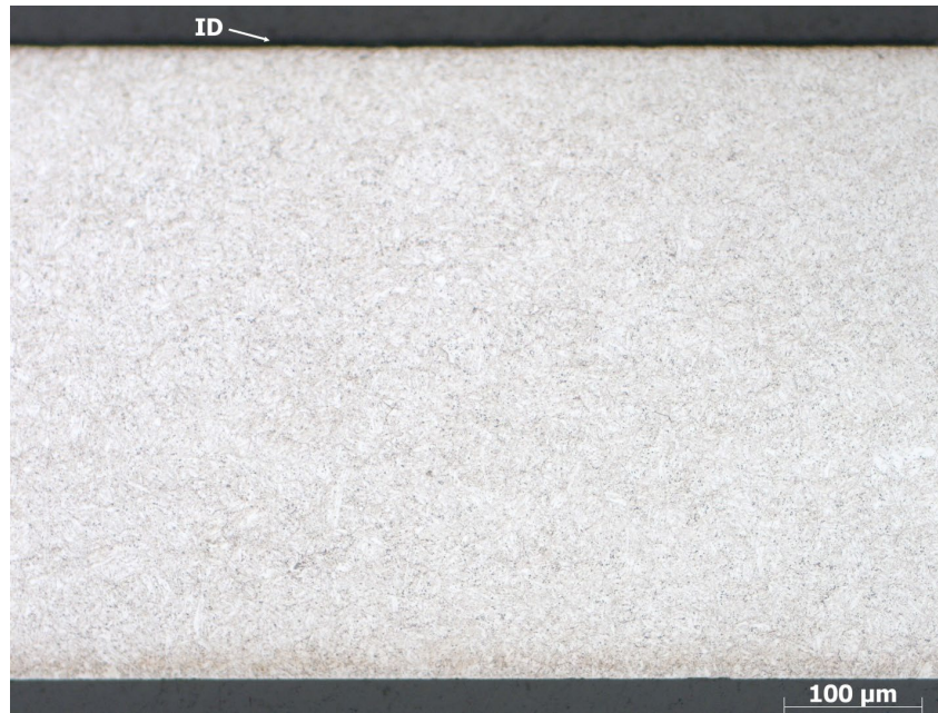
Figure 59. Area near the center of the 180° wall showing typical microstructure.
