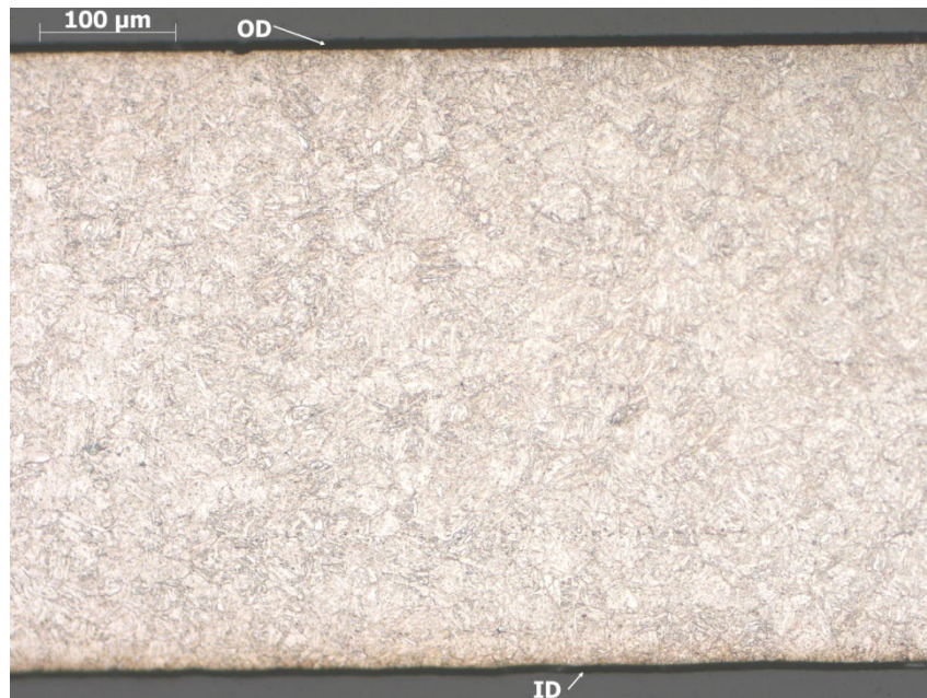
Figure 63. Lath martensite in area on the left section of the 0° wall on the EBR-II plenum section sample.
