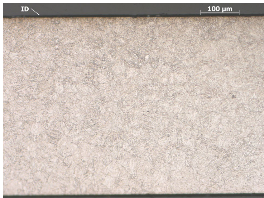
Figure 65. Area on the left section of the 180° wall showing typical microstructure.
