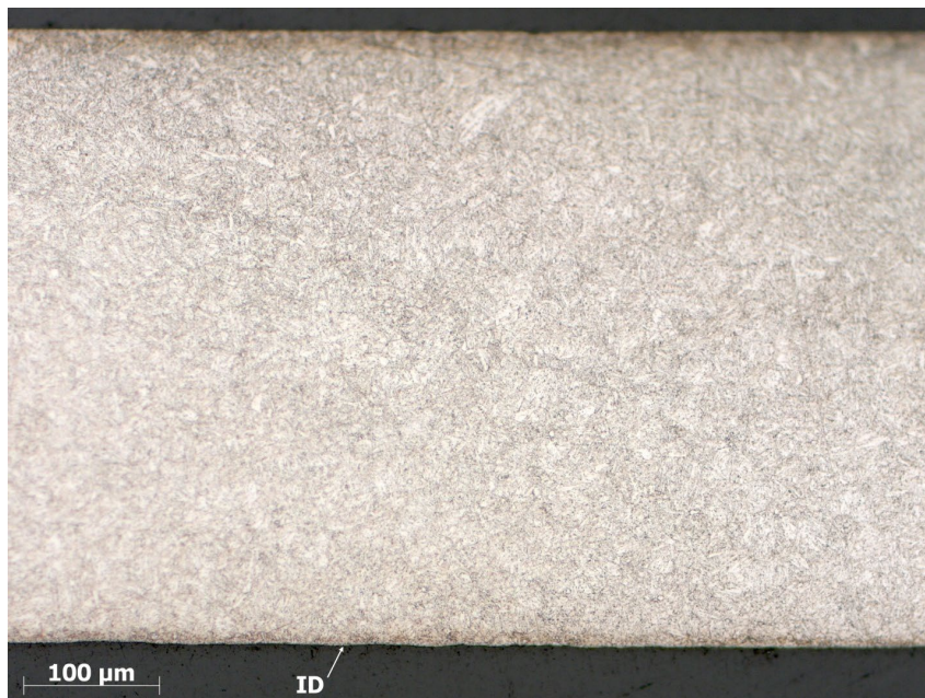
Figure 93. 0° in bright field showing lath martensite consistent with un-welded samples.
