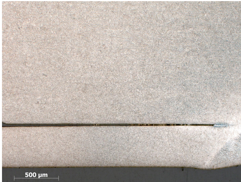
Figure 92. 180° weld showing gray tempered microstructure.
