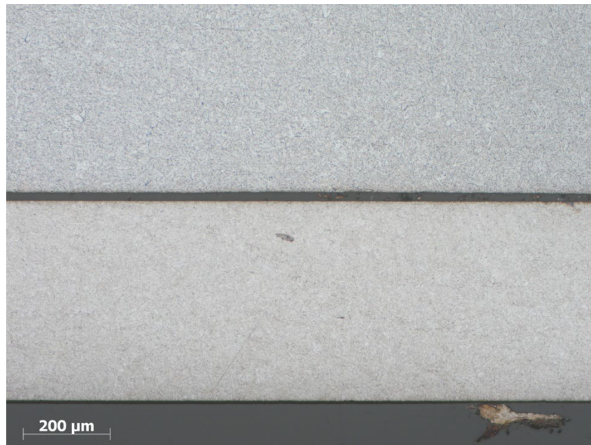
Figure 87. Area in 180° direction. Plug (top) shows gray tempered martensite while tube shows a different coloration as the initial as-drawn material or the temper conditions may have been different.
