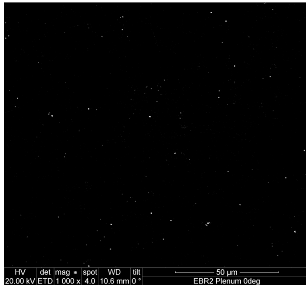
Figure 81. High-contrast BSE image of EBR-II plenum section showing the carbides as bright points.
