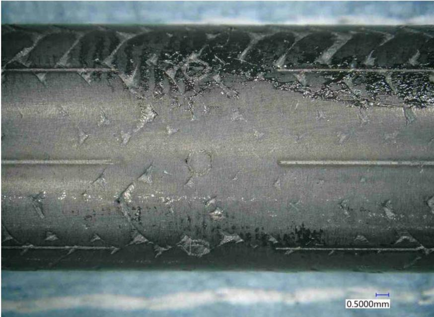
Figure 1: Close-up view of one irradiated SiC/SiC tube specimen.
