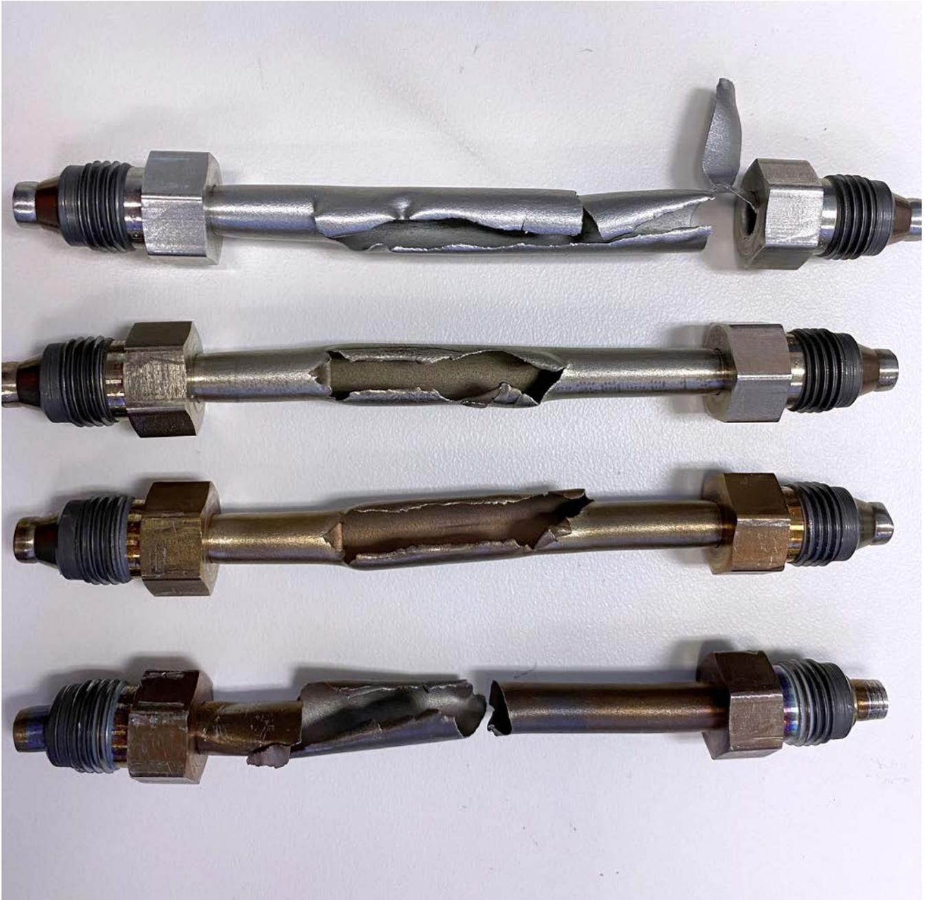
Figure 1. Photograph of tubes burst through over pressurization at different temperatures.
