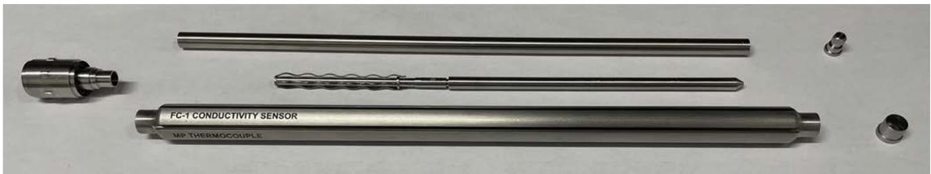
Figure 3. Completed IMPACT capsule hardware for the sodium bonded fuel capsule. Note that the fuel and sodium guard pictured is fabricated from SS316 for prototyping and assembly mockup.
