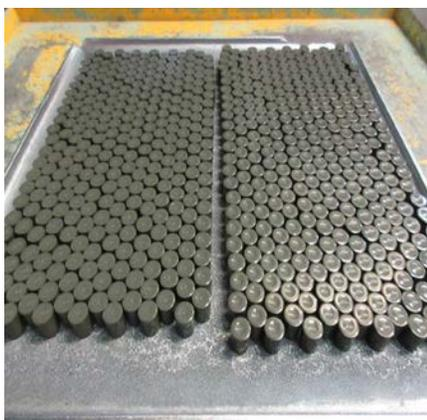
Figure 2. Low Enriched Uranium+ ADOPT pellets for loading into the Plant Vogtle-2 LTRs.
