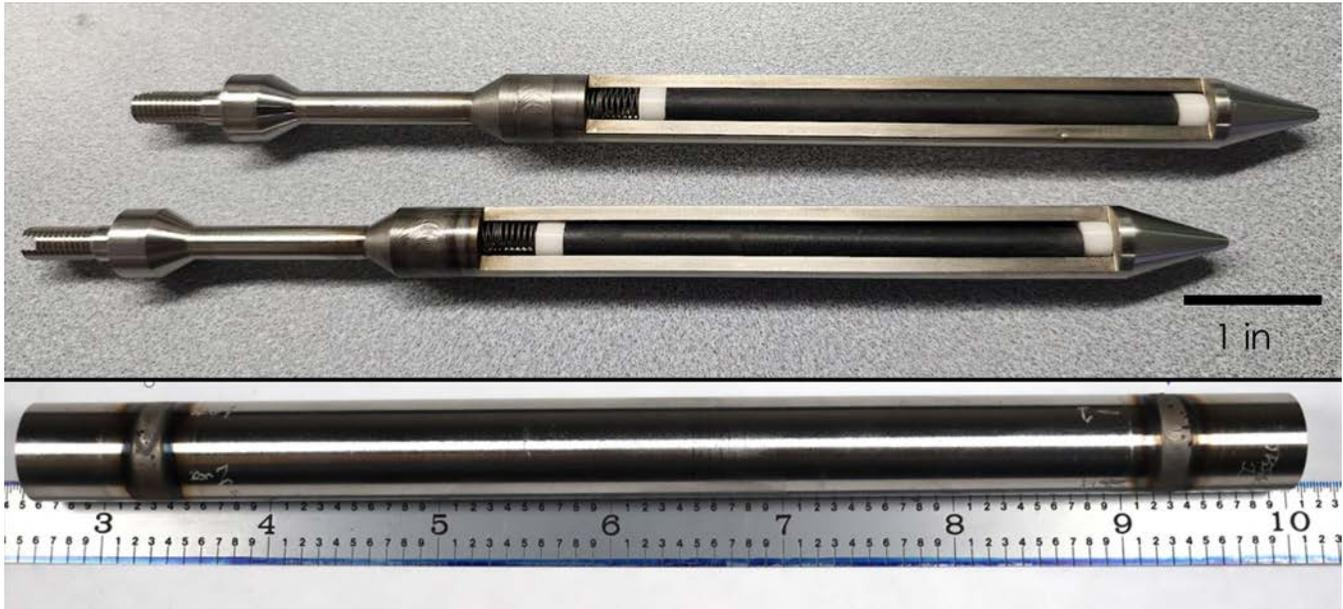
Figure 2. Innovative test vehicles have been developed and built by GA-EMS to support commercial testing of advanced in-core materials. (Top) Cutaway thimble plug irradiation capsule with SiGA<sup>®</sup> test samples prepared for commercial PWR irradiation in guide tubes. (Bottom) D capsule with SiGA<sup>®</sup> test samples for commercial BWR core periphery.
