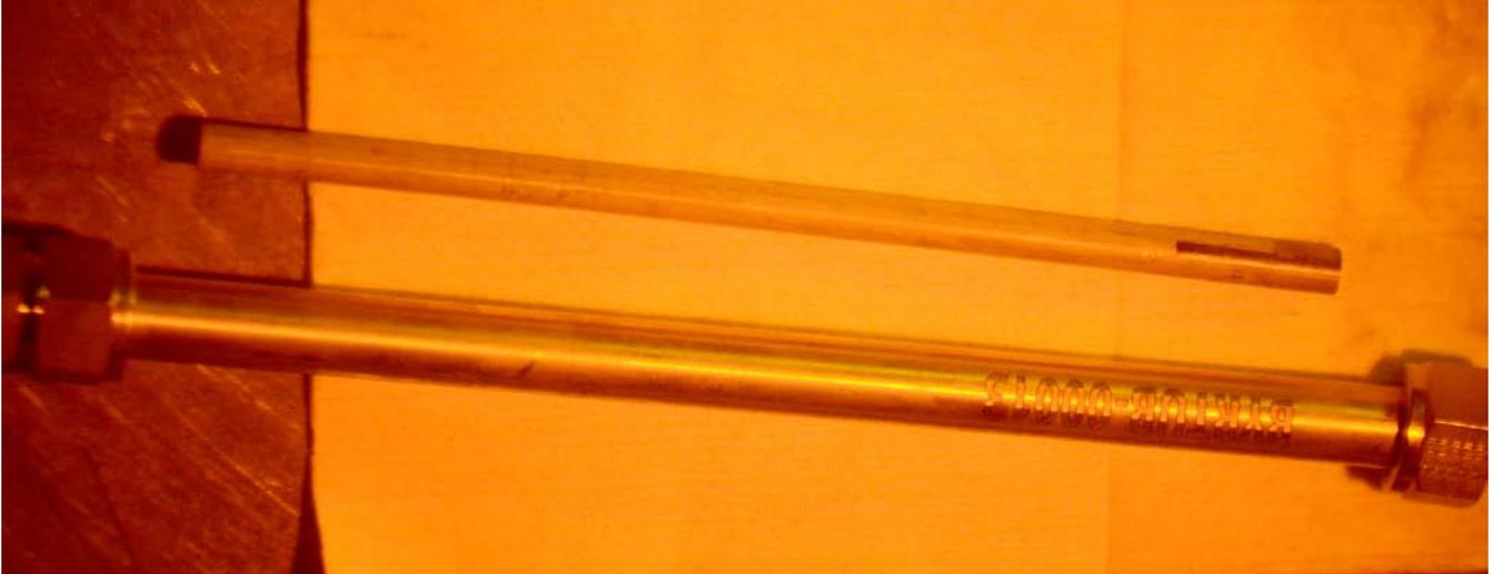
Figure 2. Segment harvested from parent rod to be used for the HERA-HBU-1 test.
