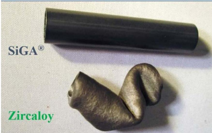
Figure 4. SiGA® brings has excellent high temperature strength for nuclear cladding applications.
