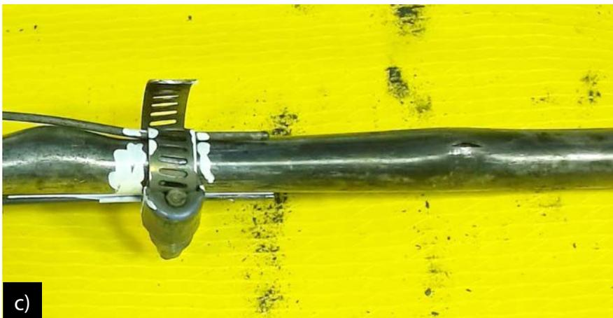
Figure 2. Post LOCA images of the NA grid spacer. a) The whole rod indicating a balloon and rupture on each side of the clamp, b) close up image of the top rupture, and c) close up image of the bottom rupture.
