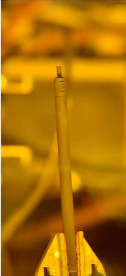
Figure 1. Visual inspections of a SiGA® rod showing no degradation after irradiation in ATR.
