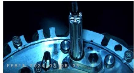
*Figure 2. Insertion the RB MiniFuel basket loaded with high-burnup targets into HFIR.*
