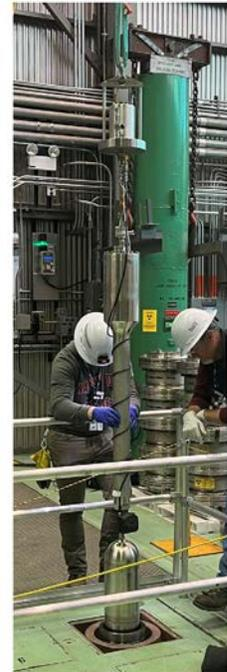
Figure 1. TWIST device configured for LOCA testing.
