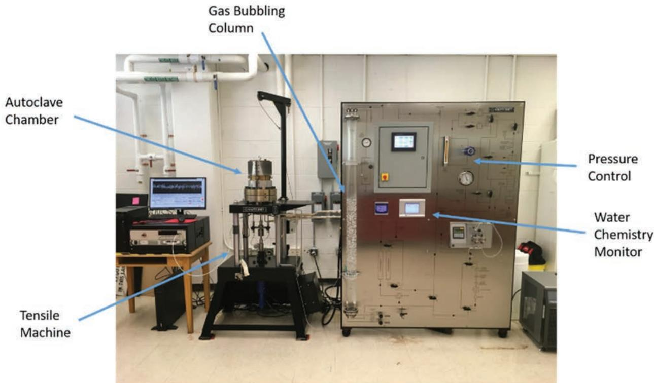
Figure 2. Autoclave setup for corrosion experiments at NCSU
