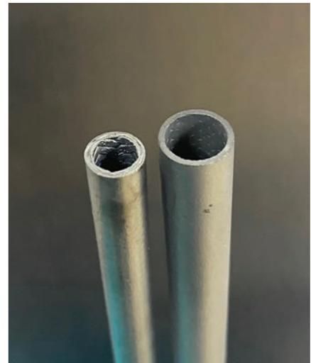
*Figure 1. Comparison of smaller diameter and standard ATF diameter SiGA® cladding*
