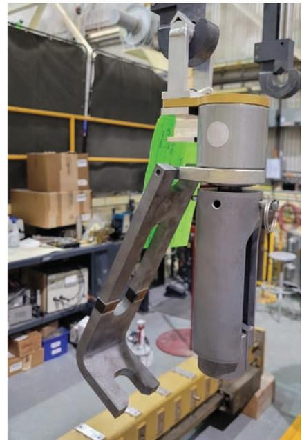
Figure 2. THOR capsule top cap torque multiplier used to seal the capsule at 120ft-lbf
