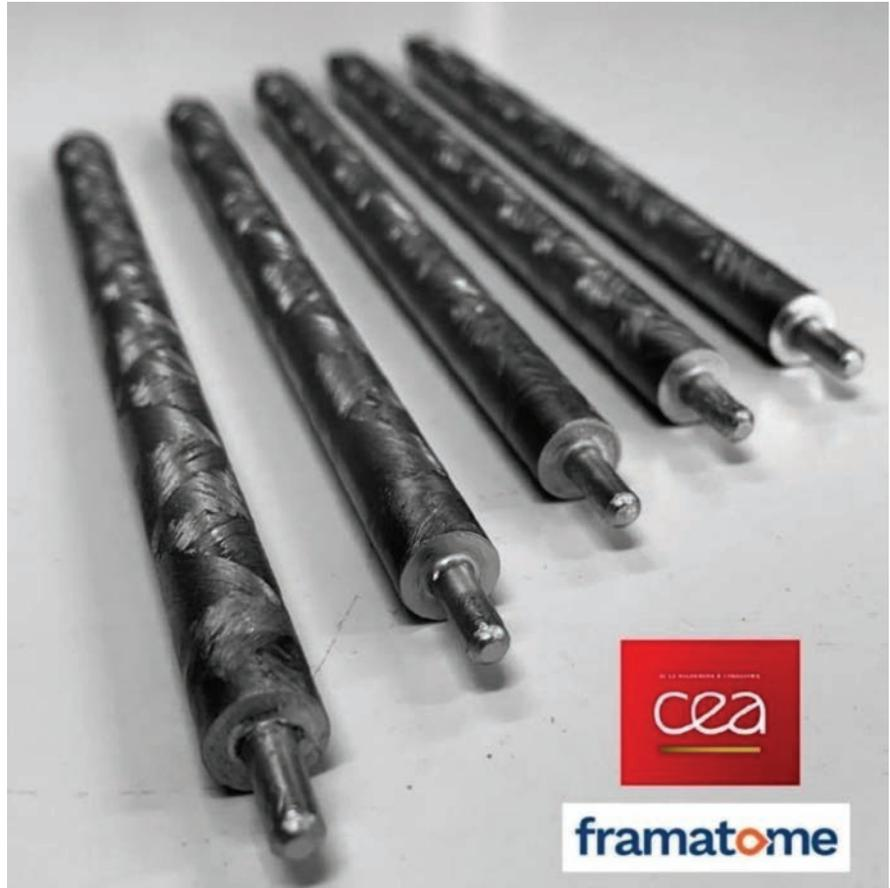
Figure 4. PROtect SiC rodlets for ATR irradiation
