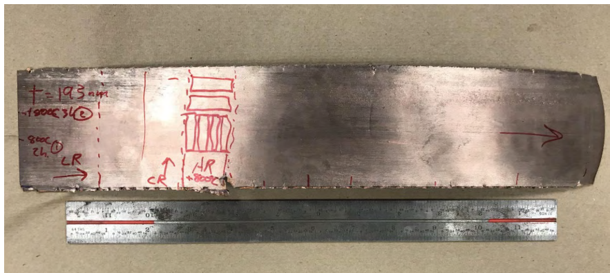
Figure 1. A photograph of the as-rolled h = 200\text{nm} ARB Cu/Nb. A ruler measured in inches is included for scale
