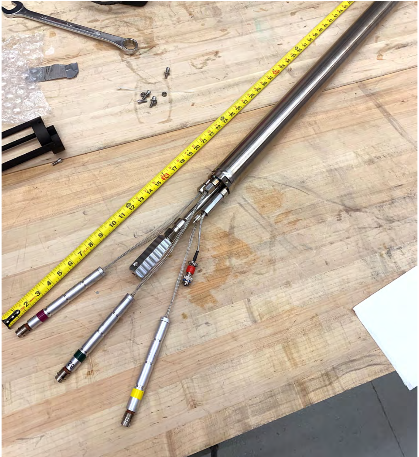
Figure 4. Assembled THOR-C-1 capsule
