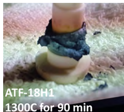
Figure 2. Images of irradiated FeCrAl after high-temperature oxidation testing at 1200°C and 1300°C for 1 minute, 15 minutes, and 90 minutes as indicated
