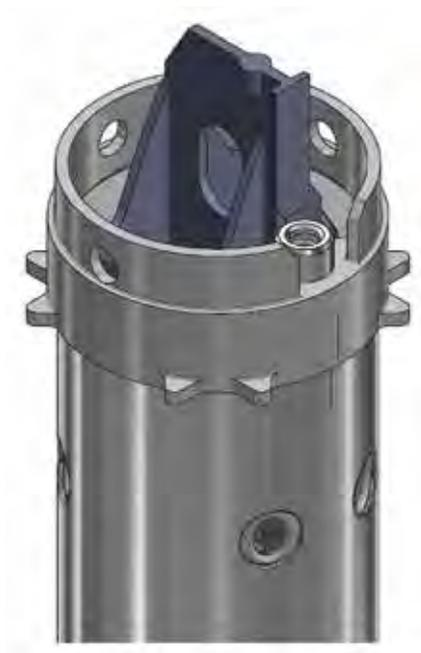
Figure 2. Booster element in holder.
