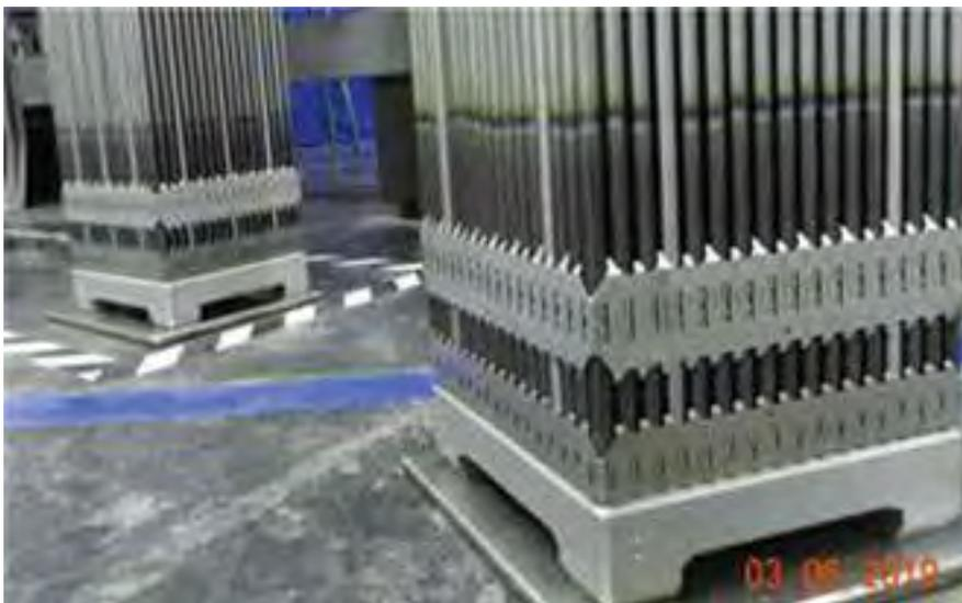
*Figure 2. Byron Unit 2 assemblies with EnCore fuel loaded.*
