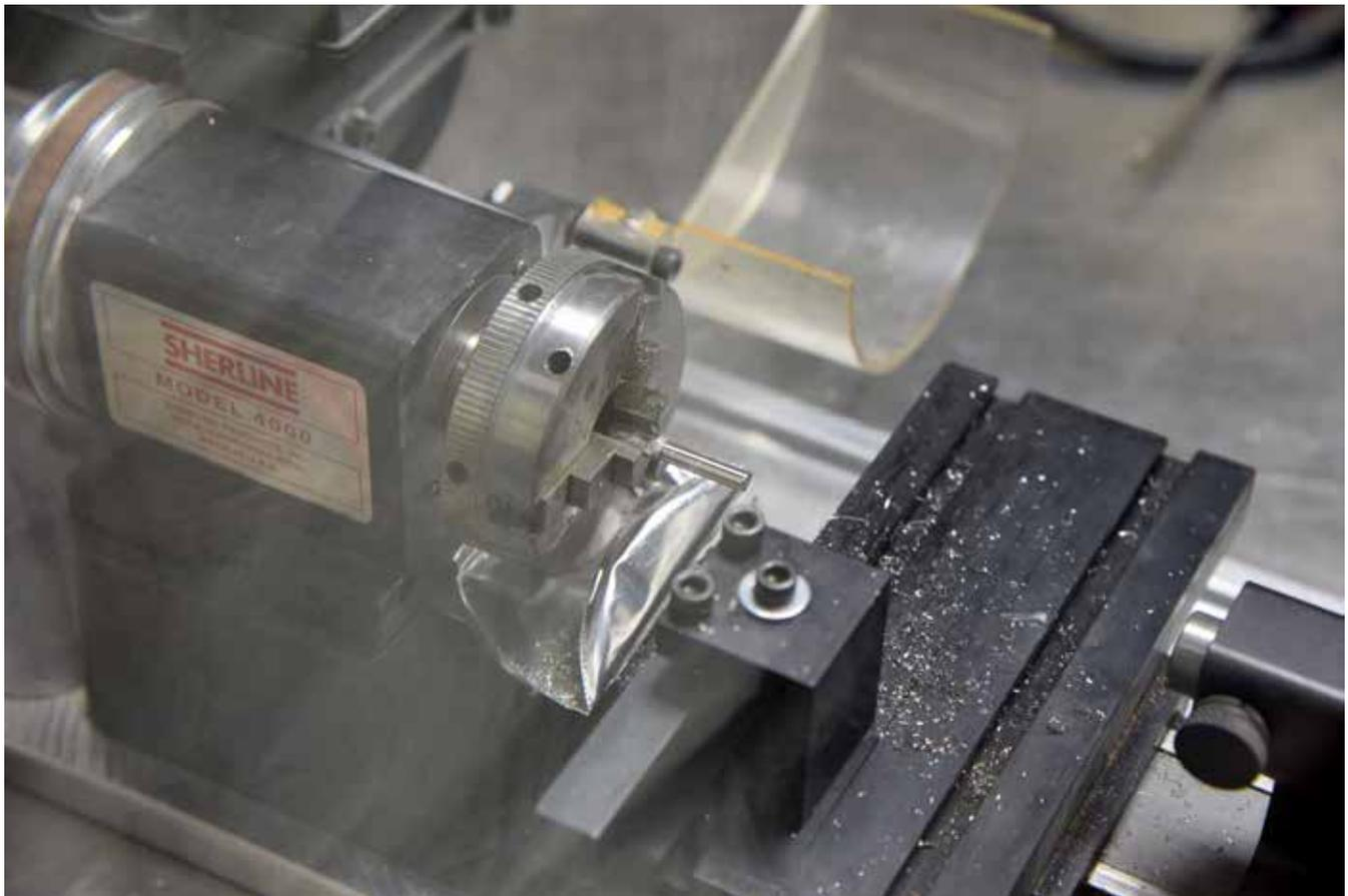
gloveboxes and equipment. A small modified hobby lathe was placed in an inert atmosphere glovebox for the process. This lathe is shown in Figure 1. The first geometry attempted was annular. This fuel geometry is of interest because the center void allows the fuel to swell inwards while
