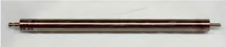
Figure 2. GE fuel rodlet for ATF-2B insertion.
