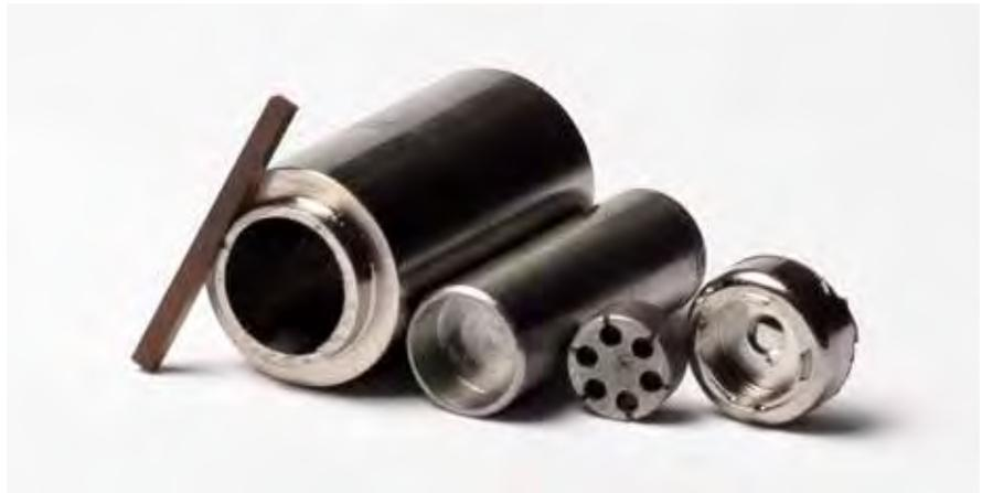
year 2021. The 6 individual capsules from the first irradiation target were extracted from the target and punctured in the Oak Ridge National Laboratory (ORNL) Irradiated Fuels Examination Laboratory (IFEL) to measure fission gas release. The kernels were then transferred to the Irradiated-Microsphere Gamma Analyzer facility within IFEL for careful extraction of the kernels and the passive silicon carbide temperature monitors, which will
