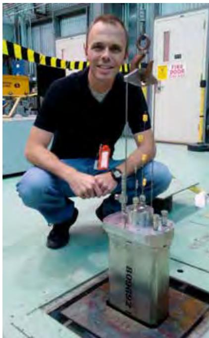
*Figure 2. First SETH capsule installed in the irradiation vehicle suspended over a storage hole at TREAT.*
