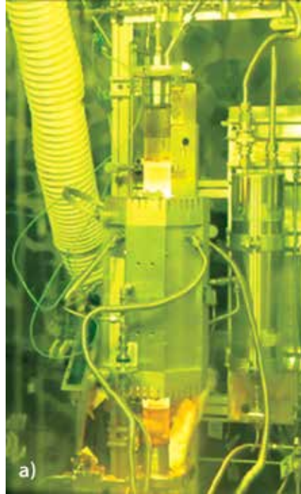
Figure 3. Photographs taken during in-cell LOCA test showing (a) the temperature ramp and (b) immediately following water quench
