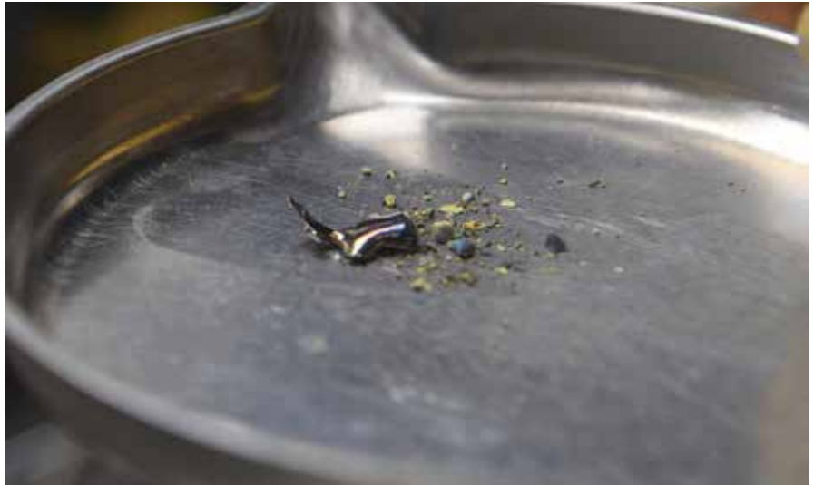
Figure 3. The same material arc melted under 4% hydrogen cover gas a second time and cooled under argon.
