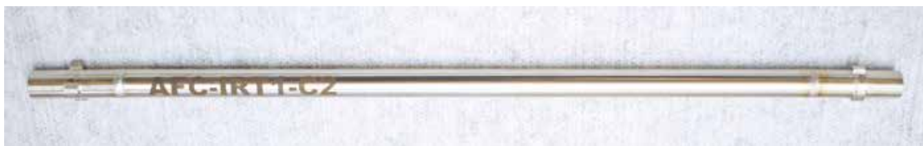
Figure 2. Typical IRT-1 capsule ready for shipment to the reactor.
