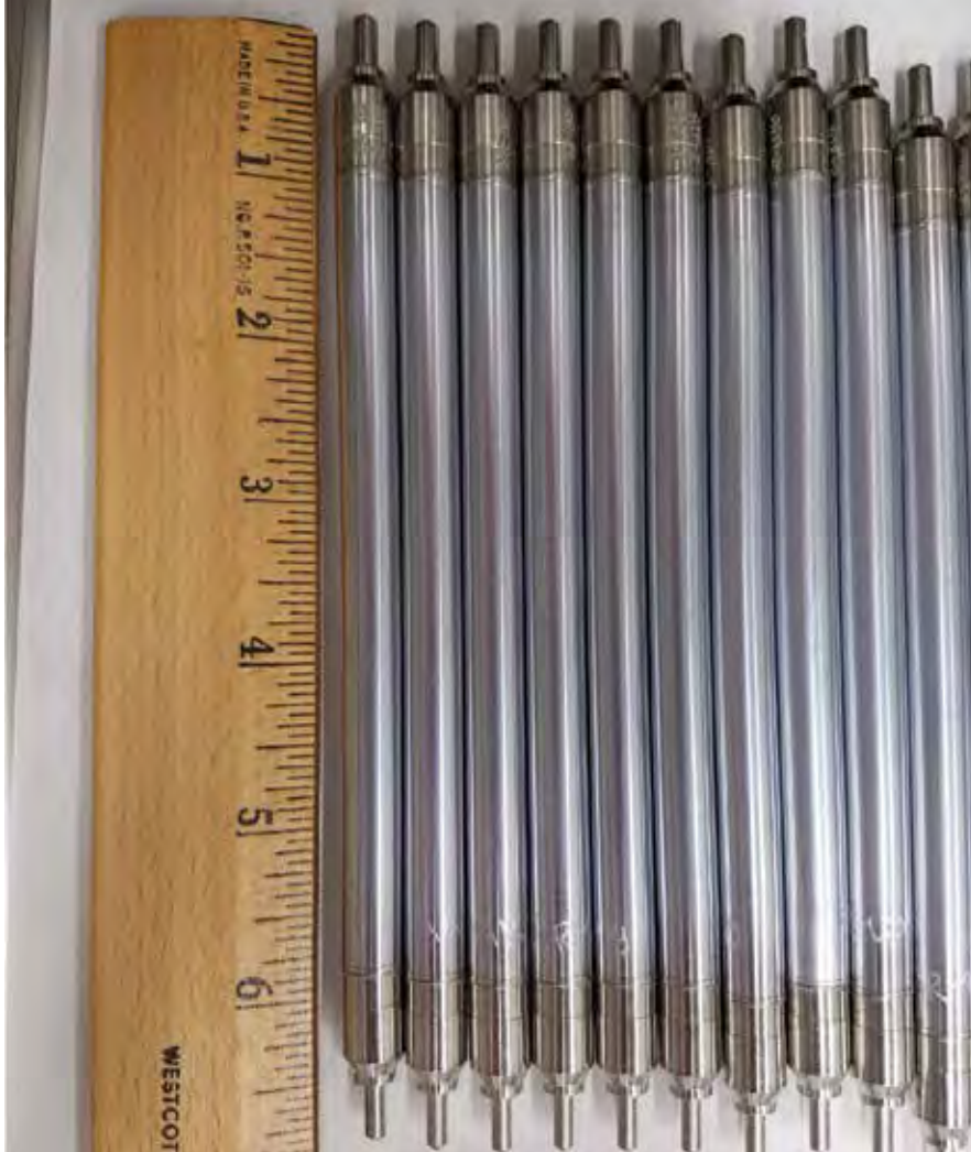
Figure 3. Cr coated cladding rodlets for ATR – ATF-2 irradiation.
