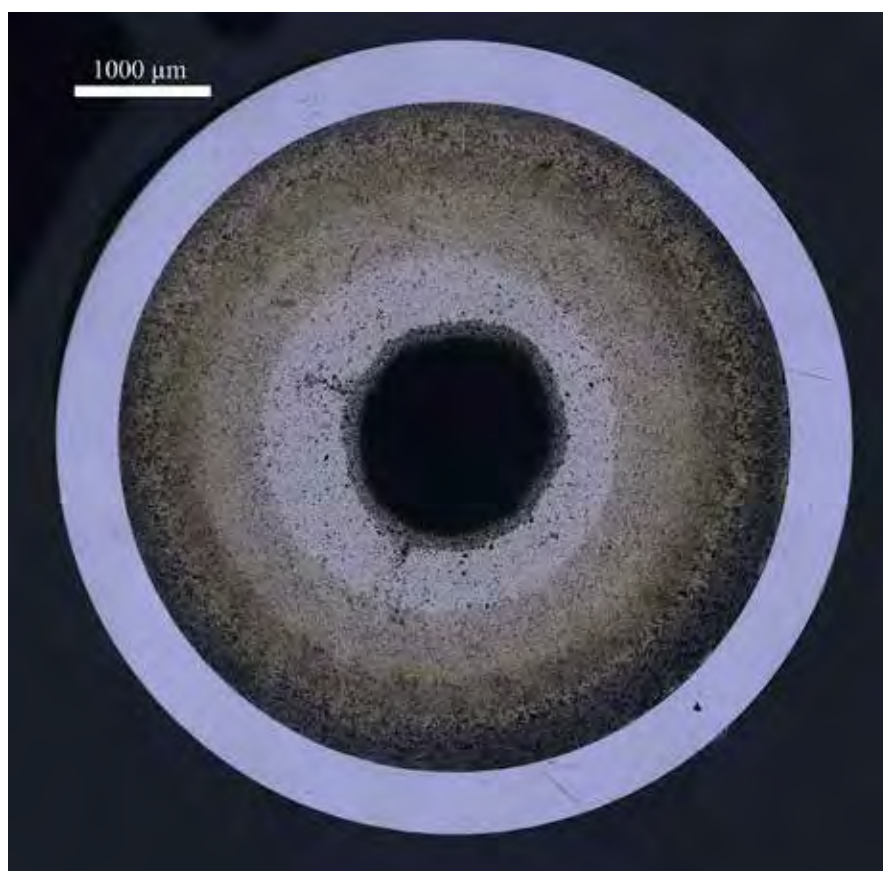
Figure 1. Transverse cross section of AFC-3D R1 (U-10Zr, 55% smear density, annular, He bonded, 4.3 atom % burnup). This fuel has performed well to moderate burnup and shows no sign of fuel cladding chemical interaction which demonstrates the need to carefully control the dimensions of fuel when using helium bonding.
