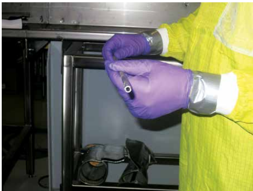
Figure 3. Annular U-10Zr produced through extrusion.
