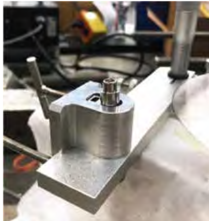
Figure 1. Cutting fixture shown loaded with a MiniFuel test sub-capsule before cutting (left) and capped for transfer after cutting (right).
