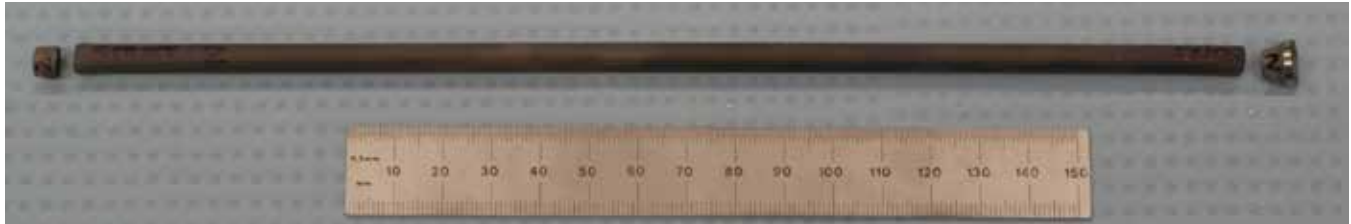
Figure 3. Image showing 14YWT tube after extrusion to 230 mm in length at CWRU using hydrostatic extrusion.
