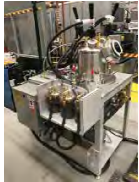
Figure 2. The new fuel fabrication line, located in the Experimental Fuels Facility at Idaho National Laboratory features an arc-melter, sintering furnace, and an inert high-density fuels glovebox.
