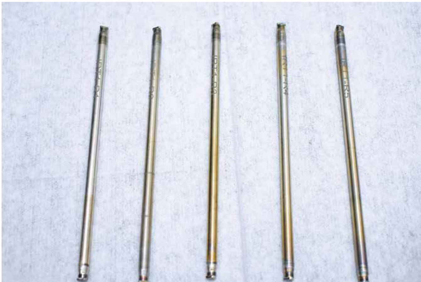
Figure 1. Completed IRT-1 rodlets ready for encapsulation.
