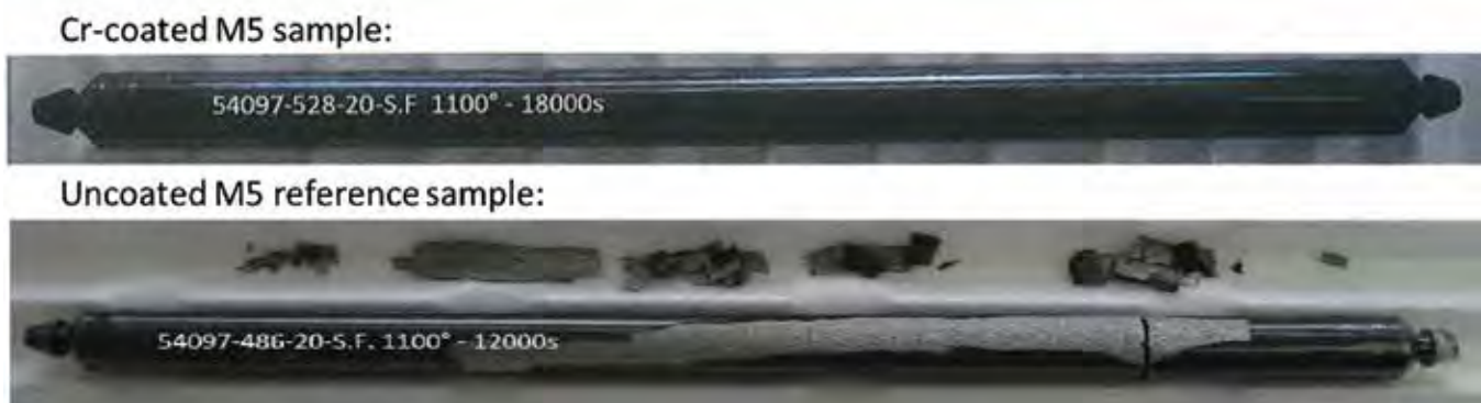
Figure 1. Photograph of cladding samples after 1100°C steam oxidation and quench: a) Cr-coated sample exposed for 18000s, b) uncoated sample exposed for 12000s.
