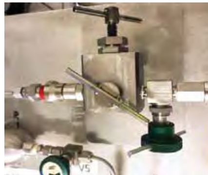
Figure 2. Fission gas puncture unit shown during testing (top left and right) and puncture tool shown after successful puncture with minimal dulling of tip (bottom).
