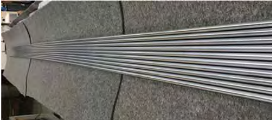
Figure 2. Full length Cr-coated zirconium-based cladding.
