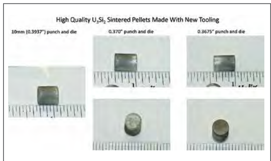
Figure 1. Improved U_3Si_2 Pellets Manufactured by INL
