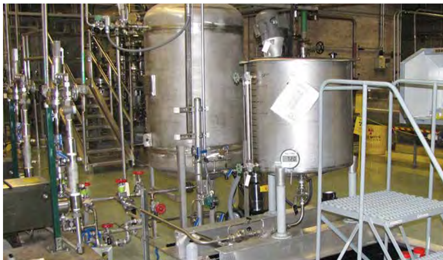
Figure 1. A picture of the boron addition system, which was developed to control boron concentrations in the loop coolant to within specified levels.
