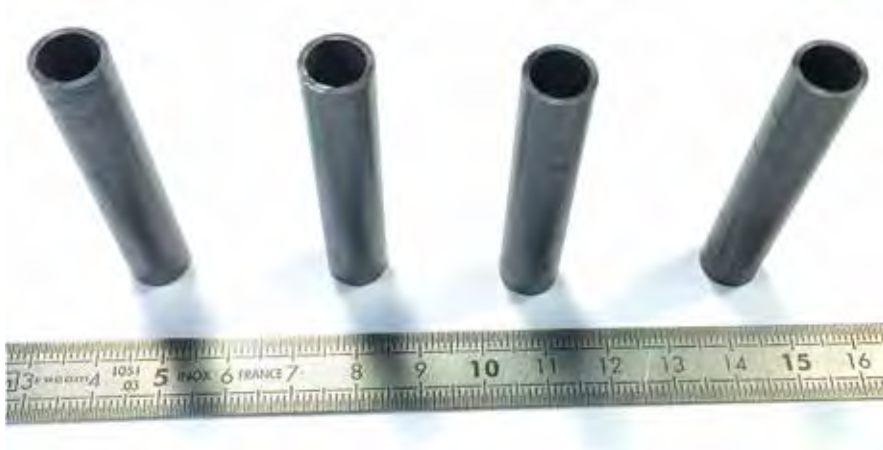
Figure 4. Samples of SiCf/SiC composite tubes (filament winding) after external / internal smoothing (© CEA).
