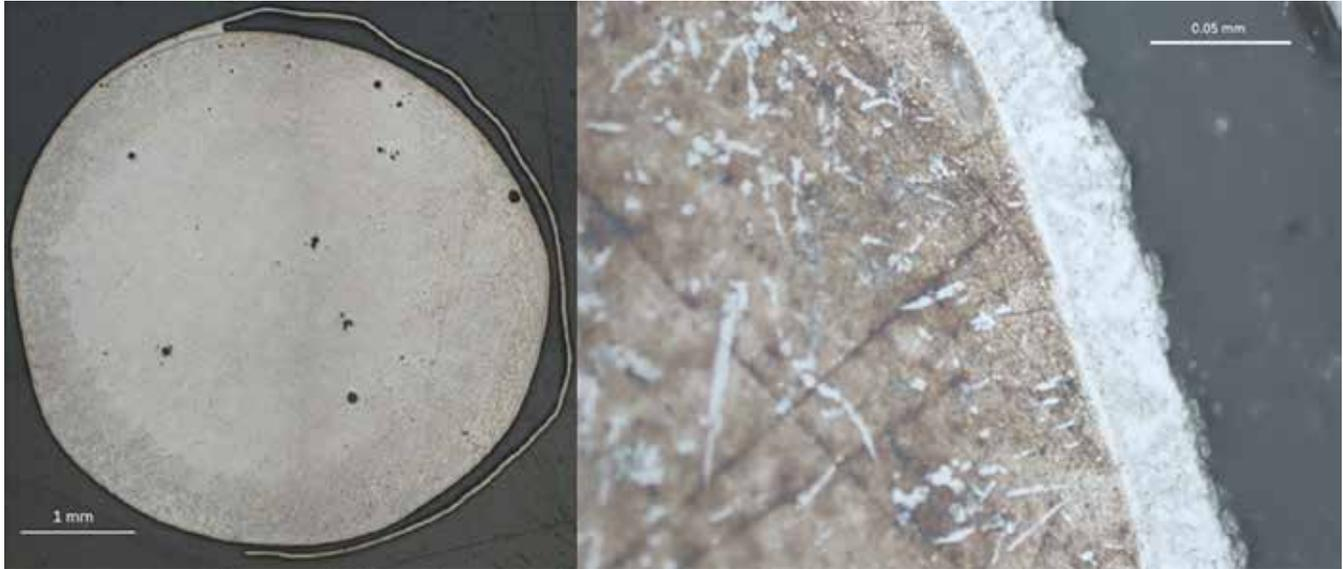
*Figure 2. Upper portion of the second attempt arc cast fuel slug.*
