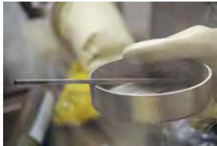
*Figure 2. Archival X521 fuel slug that was used to supply the injection cast U-10Pu-10Zr fuel slug for AFC-3F.*
