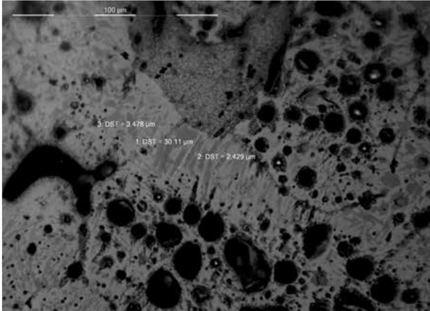
*Figure 4. Detail of phase separation present in the central region of FUTURIX-FTA DOE2*
