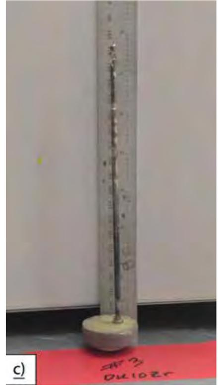
Figure 2. Typical cast rods resulting from the fluidity tests a) DU, b) DU-5Zr, and c) DU-10Zr.
