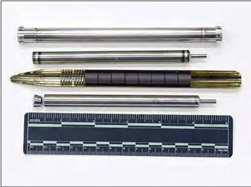
*Figure 3. From the top down: Example of ATF-1 style capsule, welded rodlet, fuel pellets, and non-welded rodlet.*
