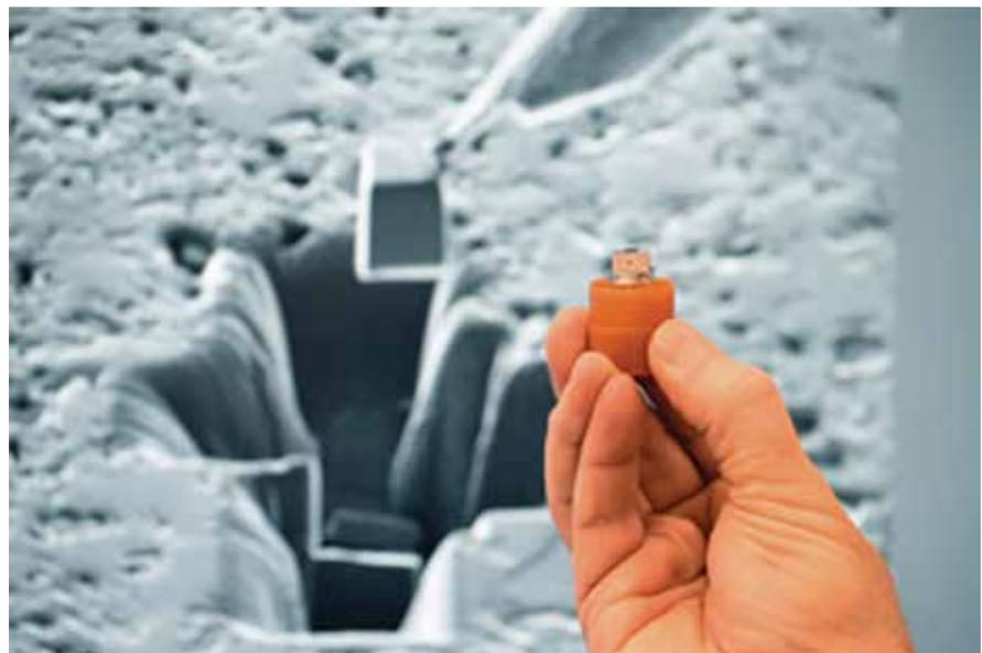
*The focused ion beam is used to remove a micron-sized cube of irradiated fuel for microanalysis. The cube is prepared as a transmission electron microscope sample mount ready to be sent for analysis.*
