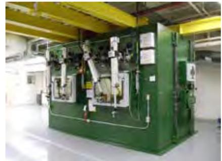
*Mechanical testing is performed in MEC-2 hotcell (right) at RPL after radioactive specimens are received and prepared for testing in MEC-1 hotcell (below). This new facility is designed to carry out highly efficient mechanical testing with temperature control in inert environment.*
