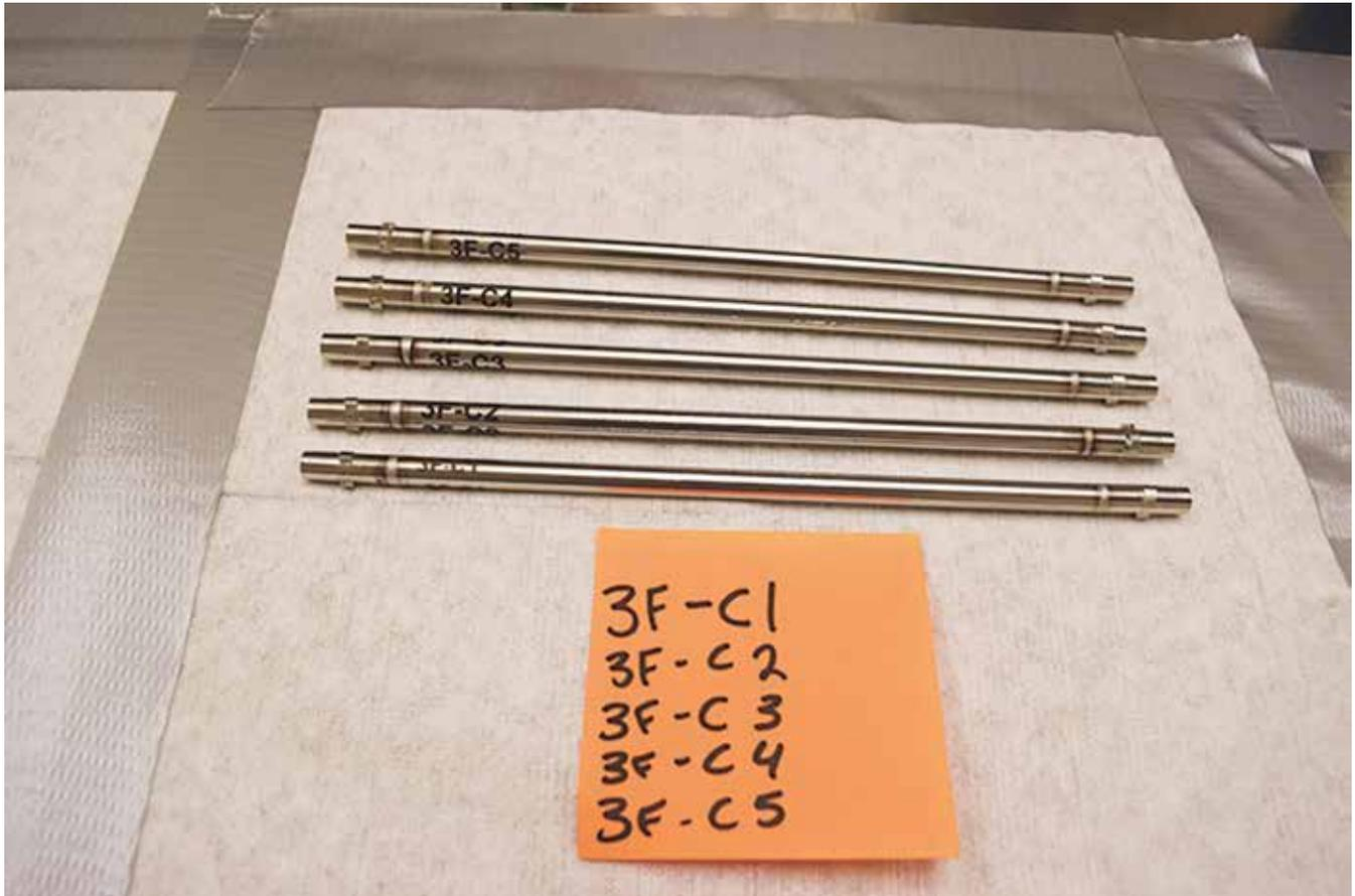
Figure 1. AFC – 3F capsules ready for reactor insertion
