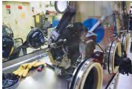
Figure 1: TRU Breakout Glovebox with 3013 can opener installed
