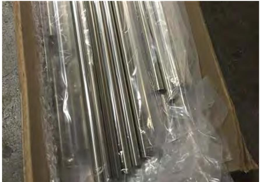
*The project has successfully established a commercial fabrication pathway of thin-wall seamless ATF FeCrAl alloy tubes which were traditionally unable to be produced because of poor deformability nature of FeCrAl alloys.*
