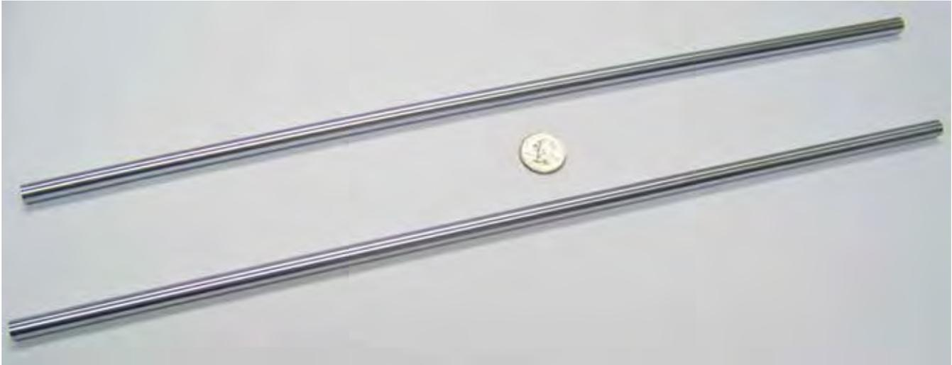
*Figure 3. 19.5 inch Long Zr-4 Tubes coated with chromium*
