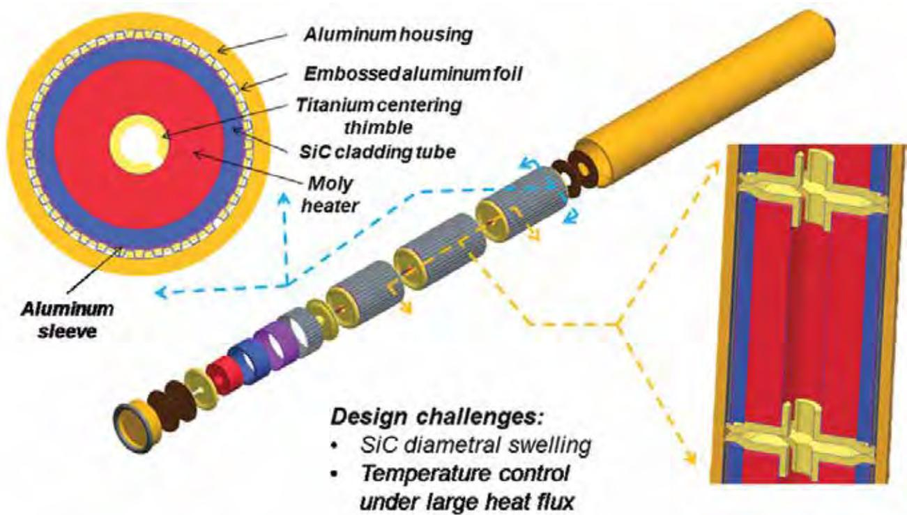
Figure 1. Illustrated design concept for innovative high heat flux "Fire Rabbit" vehicle that enabled study on the neutron irradiation – radial high heat flux synergism for development accident-tolerant fuel cladding for light water reactors.
