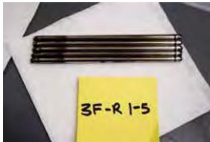
*Figure 3. AFC-3F rodlets ready for encapsulation (3F R1-R5).*
