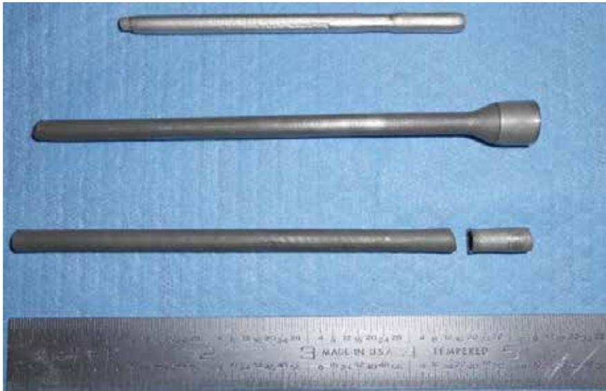
Figure 2. Multiple tubes produced by hydrostatic extrusion at CWRU on heat of 14YWT (FCRD-NFA1) shown above.
