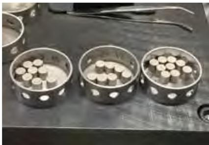
Enriched UN / U<sub>3</sub>Si<sub>2</sub> composite fuel pellets produced at FRL for ATF-1
