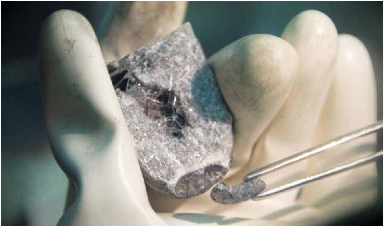
Figure 1. Metal retrieved from oxide reduction run.
