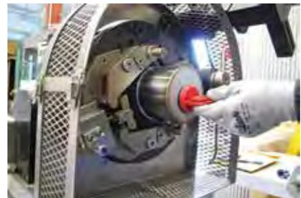
Figure 4: Inner nested can of 3013 mock-up set being removed from outer can
