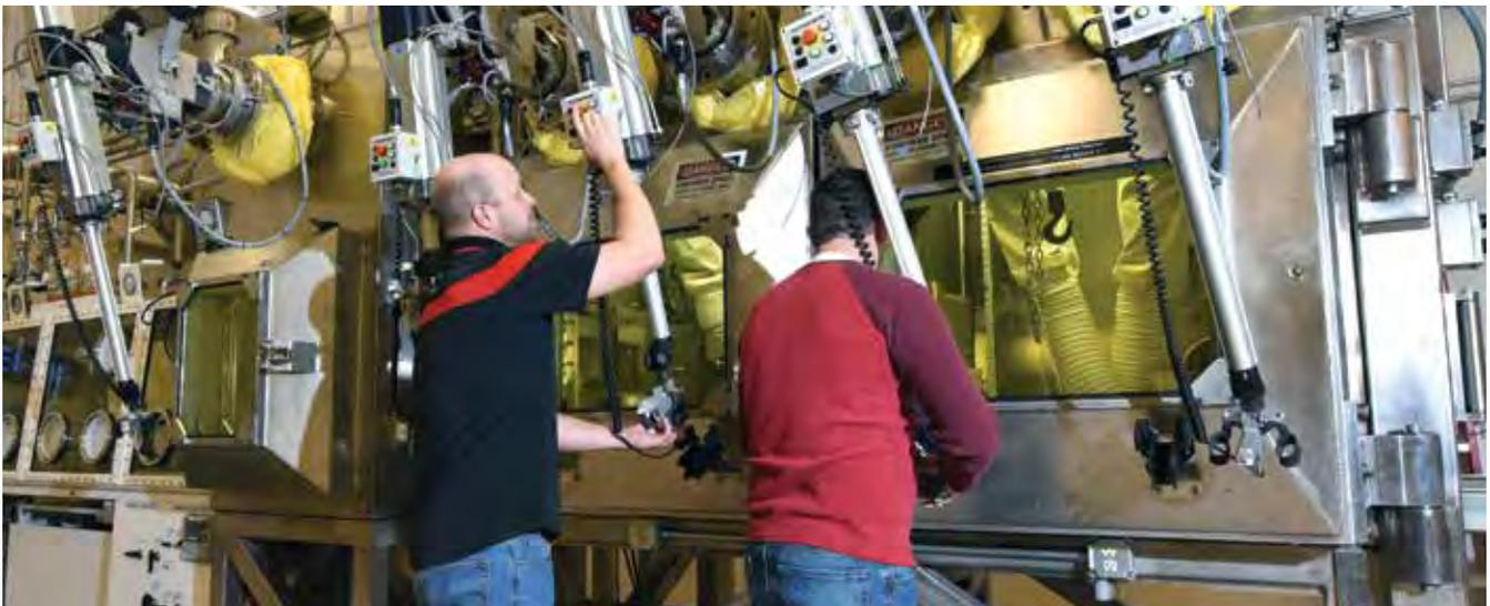
*Irradiated materials are prepared for examination right to left: the Shielded Sample Preparation Area (SSPA), the Shielded Transfer Cell (STC), the glovebox, and the fume hood*
