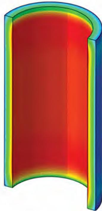
*Figure 2. Stress distributions in SiC/SiC tube after cooldown to room temperature following ~2 dpa irradiation in Fire Rabbit experiment for study on the neutron irradiation – radial high heat flux synergism, estimated by a multi-physics finite element analysis.*
