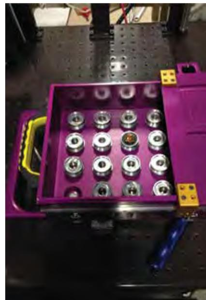
*This radiation-shielded magazine safely holds samples for analysis*
