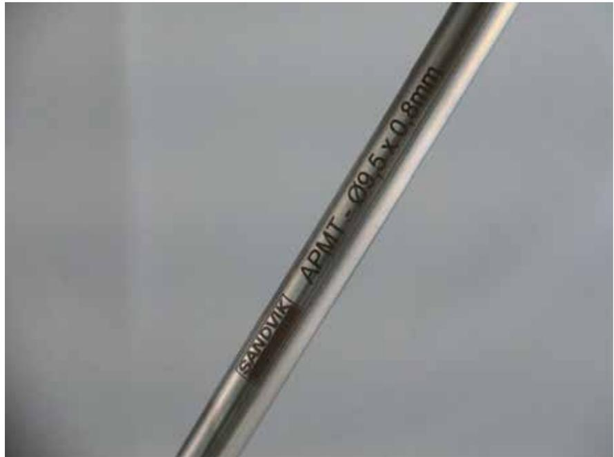
The General Electric (GE) accident tolerant fuel (ATF) design concept utilizes a FeCrAl alloy material as fuel rod cladding in combination with uranium dioxide (UO<sub>2</sub>) fuel pellets currently in use, resulting in a fuel assembly that leverages the performance of existing/current LWR fuel assembly designs with improved accident tolerance. The use of FeCrAl cladding is a direct near term path to improve the safety of operating commercial light water reactors.
