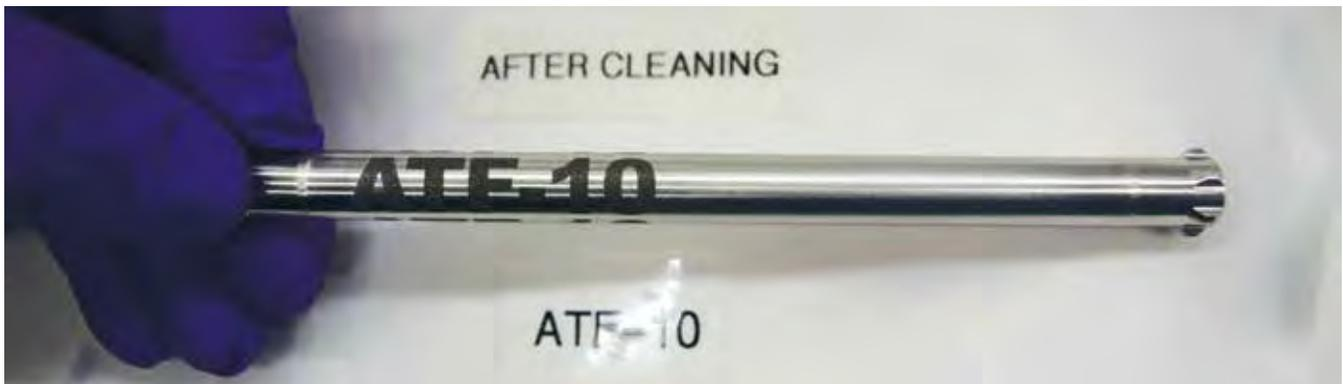
Figure 1. U<sub>3</sub>Si<sub>2</sub> Fueled Rodlet Now In ATR
