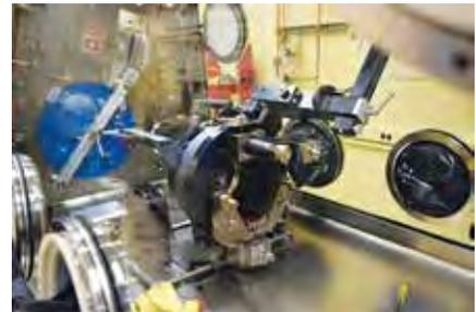
Figure 2: TRU Breakout Glovebox with 3013 can opener installed
