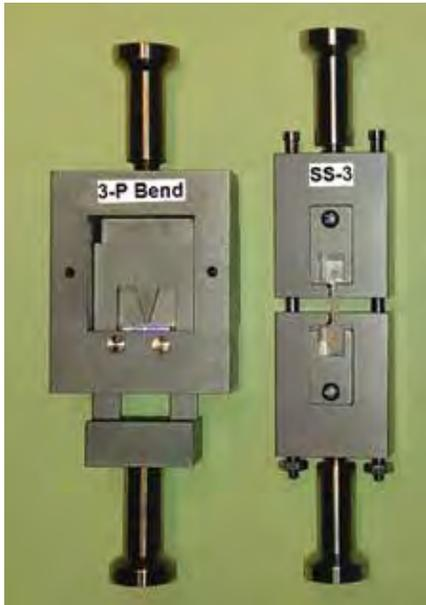
*Inside the test frame in MEC-2 hotcell: A cradle-type fracture testing grip is loaded on the load train (left) with the three-zone furnace opened. Two mostly used testing grips are shown below, respectively for three-point bend fracture testing and uniaxial tensile testing.*
