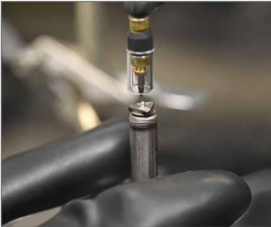
*Figure 2. Micro-TIG torch setup in inert atmosphere glovebox for closure weld of weep hole on ATF rodlets.*
