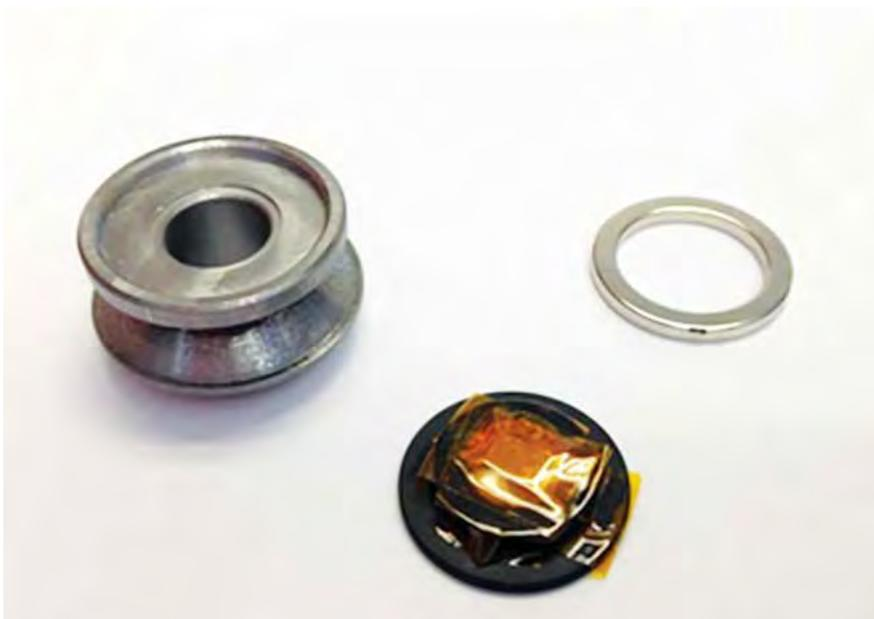
*Holder with magnetic closure ring for rapid loading of radioactive samples*
