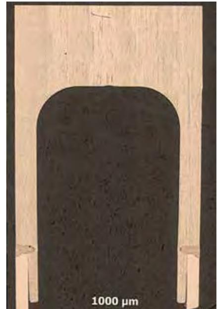
*Figure 2. Example endplug welded as part of laser welder demonstration; material is SS316L.*
