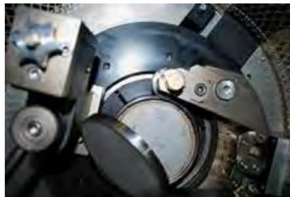
Figure 3: 3013 Can opener cutting the outermost container of a 3013 mock-up set
