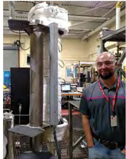
*Figure 2. Autoclave at the Westinghouse Research Laboratory to be used to examine sensor and cladding durability under prototypic PWR and ATR flow conditions prior to ATR insertion.*
