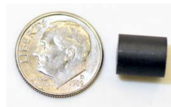
Figure 65. ATF Fuel Pellet
