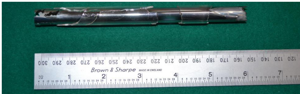
Figure 61. Photograph of a 6-in.-long free-standing Mo tube produced via the FBCVD process.
