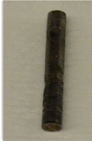
Figure 26. Photo of U-10Zr transmutation fuel with 5% rare earth (lanthanide mix) rare earth inclusion.
