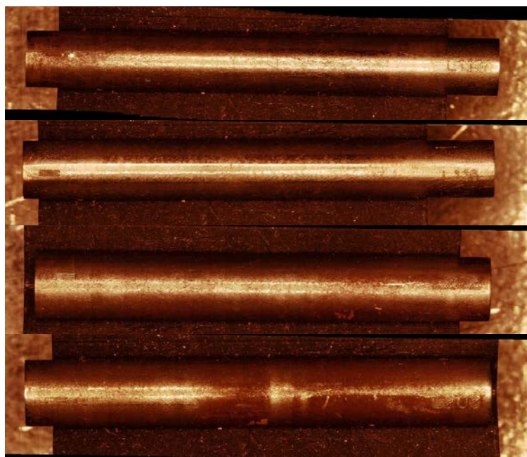
Figure 100. NFA1 tubes after cleaning, imaged at 20x, showing discoloration and corrosion. Sample IDs are clear, from top: L110, L116, L202, L203.
