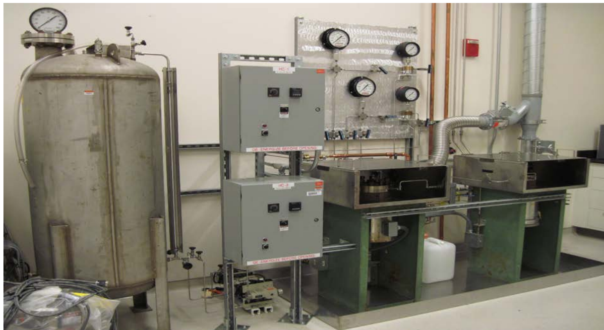
Figure 42. Installed U-Mo Metal-Water Testing System Capable of Operating at PWR Conditions.
