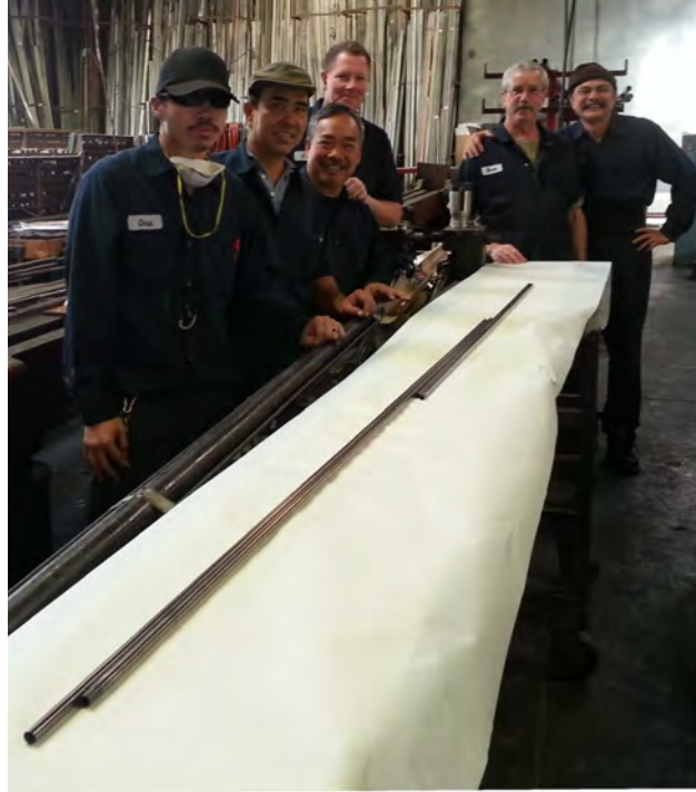
Figure 40. Photo showing tubing produced from Phase 1 FeCrAl alloys by Century tubing (from left to right, Chris Truong, Vincent Le, Ly Pham, Joe Carr, Dave LaBerge and Dan Tran).
