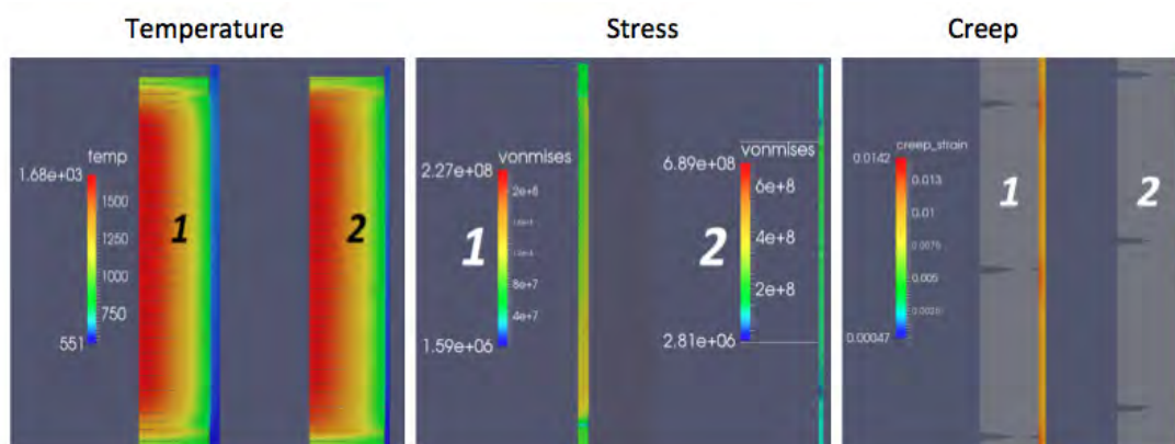
Figure 17. Zircaloy(1) and APMT 0.5(2) Hot Condition Full Rod Temperature, Stress, and Creep Results
