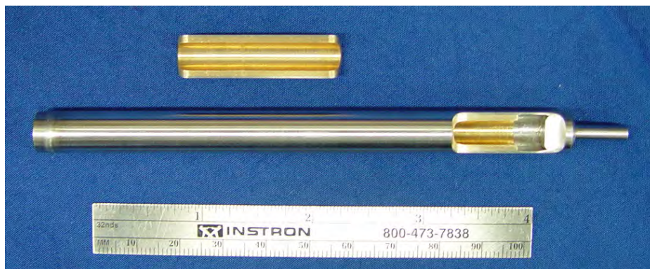
Figure 29. Finished model rodlet with machined viewing windows.
