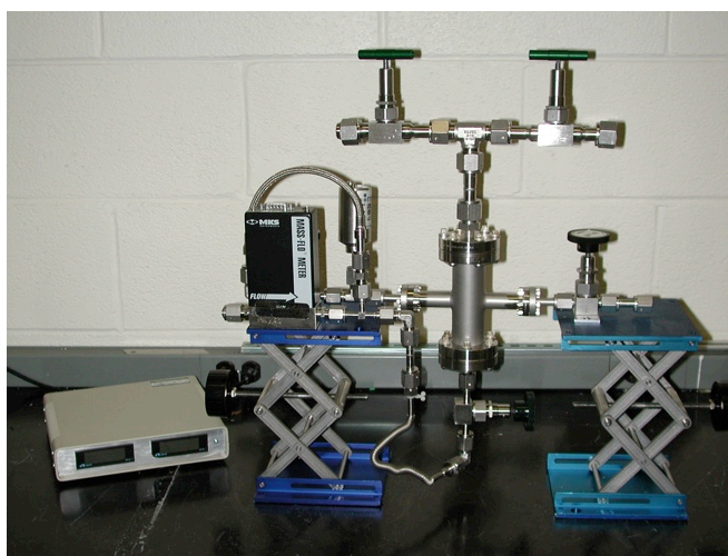
Figure 13. UF_6 Deconversion Lab-scale Reactor Vessel
