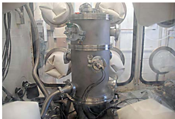
Figure 29. Glovebox Advanced Casting System installed and assembled in the Casting Laboratory glovebox.
