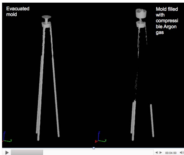
Figure 42. A snapshot of casting with and without argon at 4.5 seconds.
