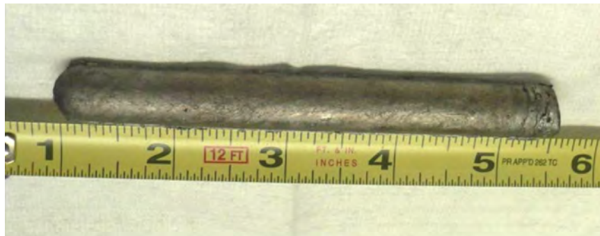
Figure 15. Typical example of cast product for TEM disc preparation (scale is in inches).
