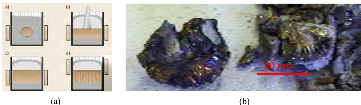
Figure 78. (a) Illustration of skull melting process illustrating melting in the center of the powder, powder filling into melt, full melt and nucleation and growth of grains; (b) zirconia crystals formed from skull melting test.
