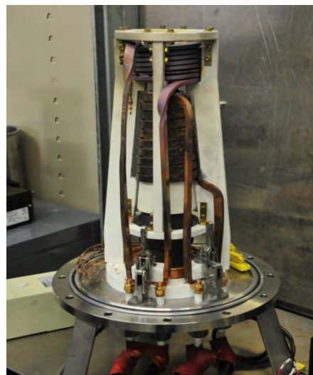
Figure 23. GACS internal components and support structure.
