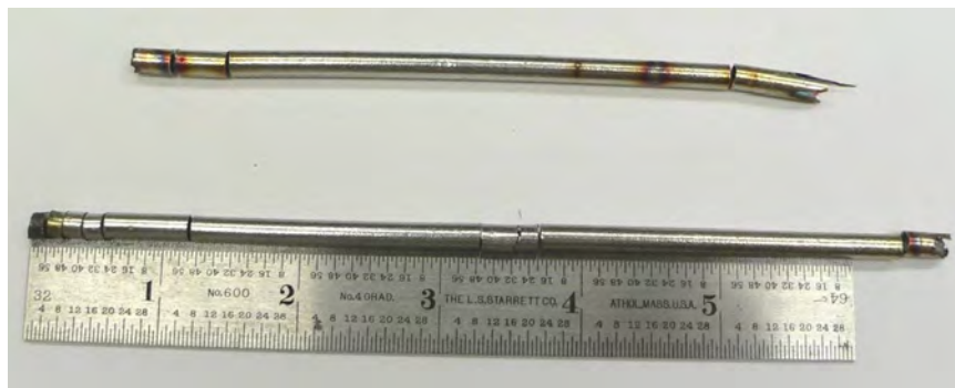
Figure 19. Typical examples of the “straws” cast without use of an inner core.
