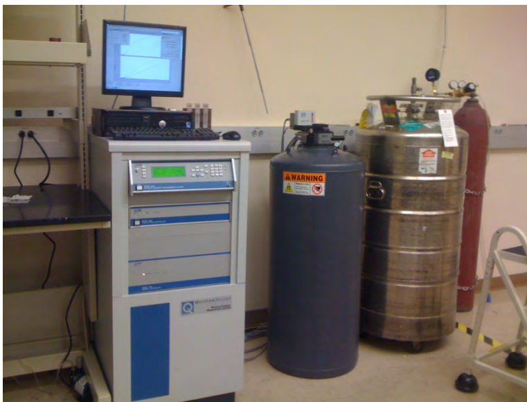
Figure 42. The Physical Properties Measurement System (PPMS) at UNLV. During measurement, the sample resides in the dark gray Dewar near the center of the photograph.
