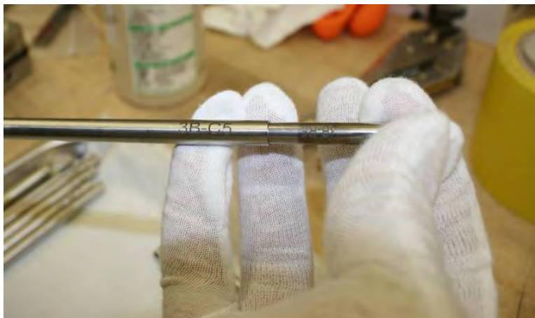
Figure 25. Verifying rodlet serial numbers and inserting rodlet into capsule.
