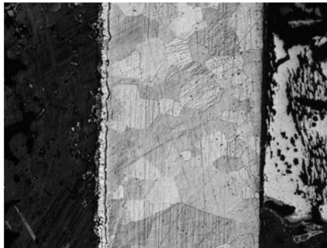
Figure 56. SEM of diffusion couple: Nd / Fe / Pd-Nd alloy (materials, left to right) illustrating benefit of intermetallic formation between palladium and neodymium. The diffusion couple was heated at 700oC for 100 hours, and the double reaction zone is apparent on the left.
