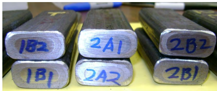
Figure 104. The coupons cut from the extruded bars. Note that in the coupons the inner meat part is the NFA and the outer rim part is from the carbon steel can.
