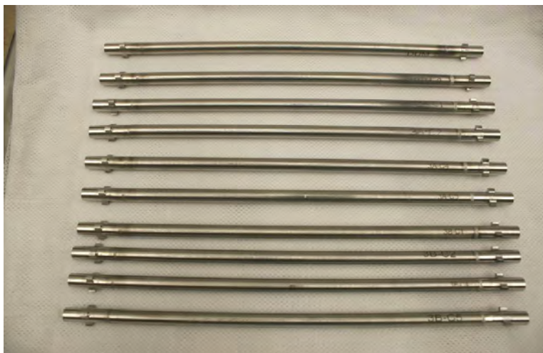
Figure 27. Finished capsules loaded and welded.
