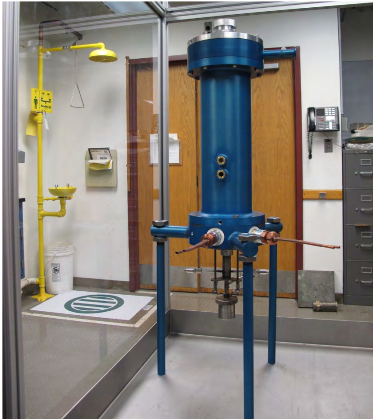
Figure 86. Photograph of the new particle coating furnace.
