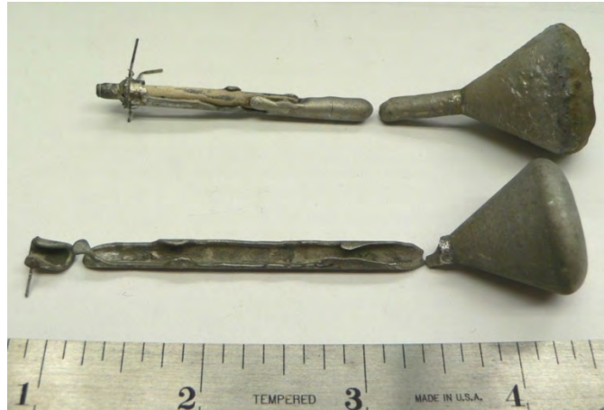
Figure 18. Examples of casting results using a Vacuum Pressure Casting Machine.
