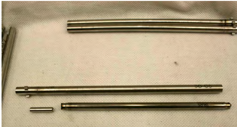
Figure 24. Rodlets and spacer laid out for loading into capsule.
