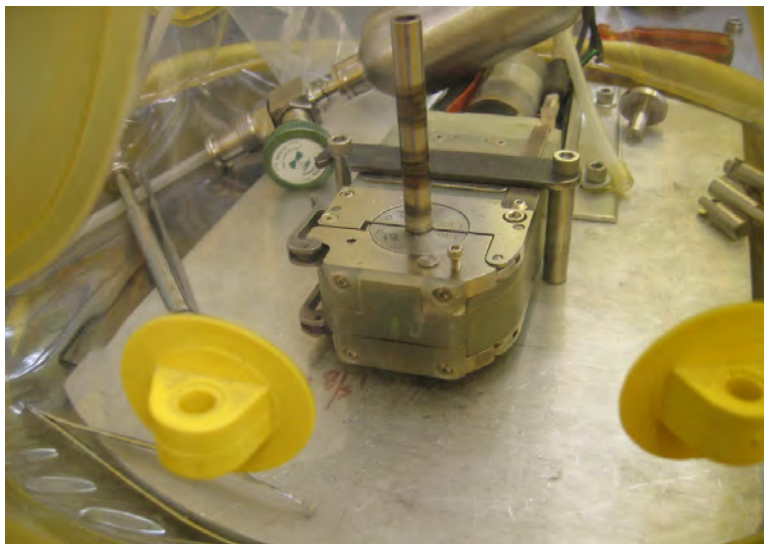
Figure 26. Orbital welding system used for capsule closure weld inside a He glove bag with a test weld piece shown in place.
