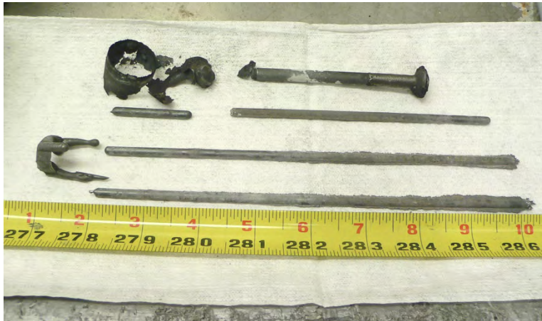
Figure 8. Result of BSC casting with argon initially in the mold. Each rod cavity is 10 inches long. Photo courtesy of Randall Fielding, INL.
