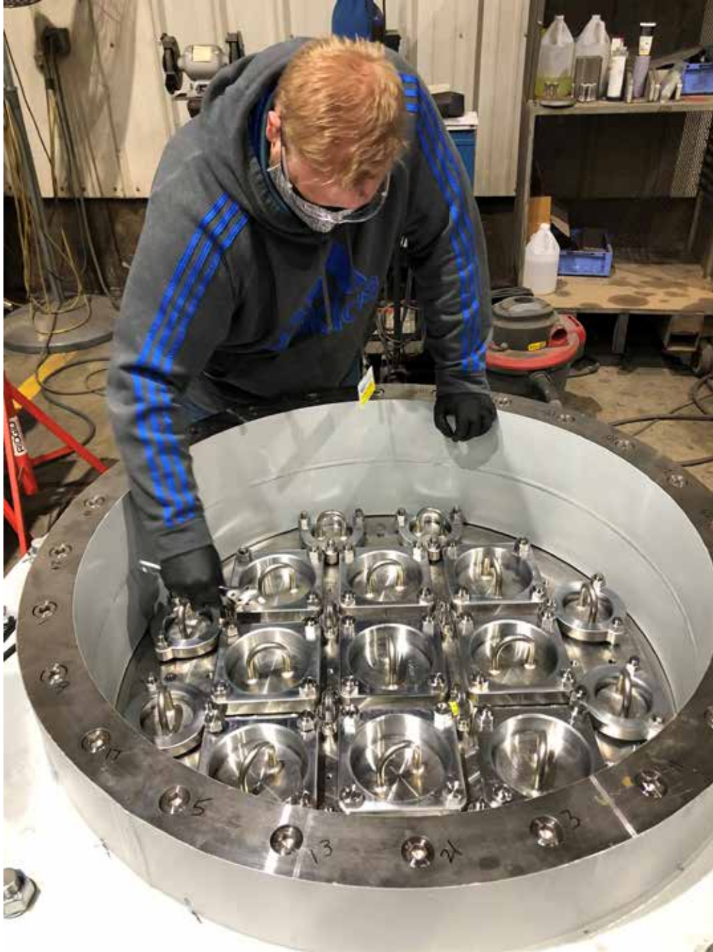
Figure 5. Mark II hydro testing assembly (Nate Oldham)
