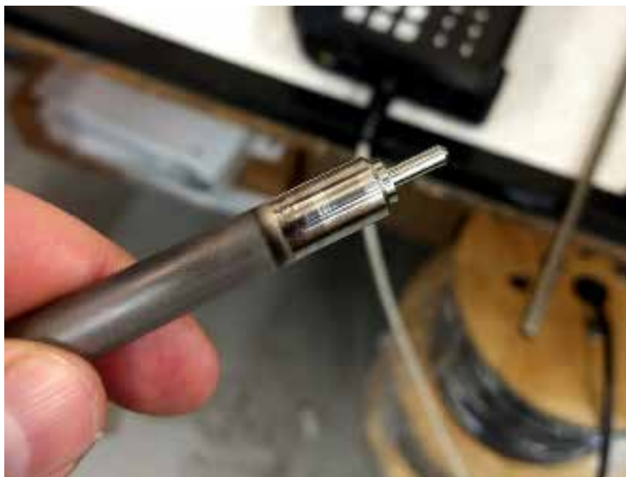
Figure 4. Successful weld demonstrated on oxidized cladding during out of cell testing of circumferential welder
