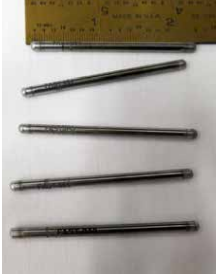
Figure 2. Assembled FAST rodlets. Each rodlet contains a 0.75" long fuel pin that is scaled at \frac{1}{2} of the radius of standard Experimental Breeder Reactor (EBR-II) or AFC fuel pins. Each capsule can hold up to two of these rodlets, notionally a standard U-10Zr control rodlet and one of the novel fuel designs to be tested.
