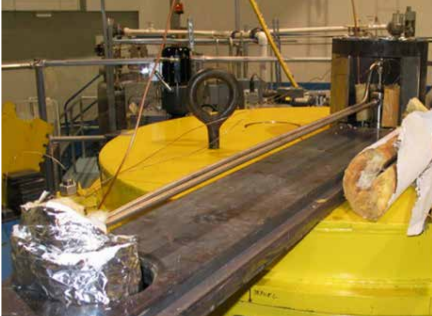
Figure 3. Images of MITR's water loop and cladding test holder
