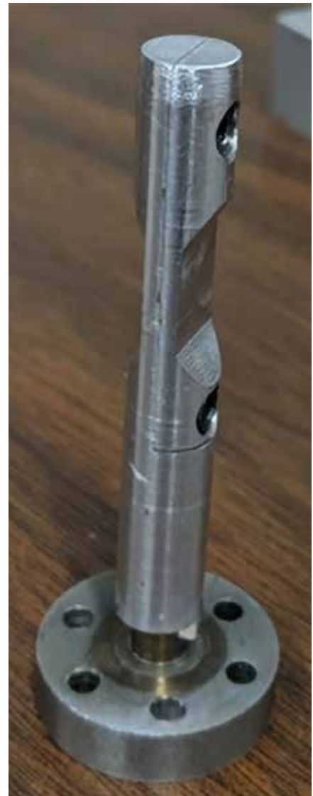
Figure 1. Opened aluminum sample holder with the cavity for the disk of irradiated U-10Zr-1Pd in the thinned section marked by an arrow (left). Sample holder closed and attached to the lid of a vanadium can that provides secondary containment of the sample (right).
