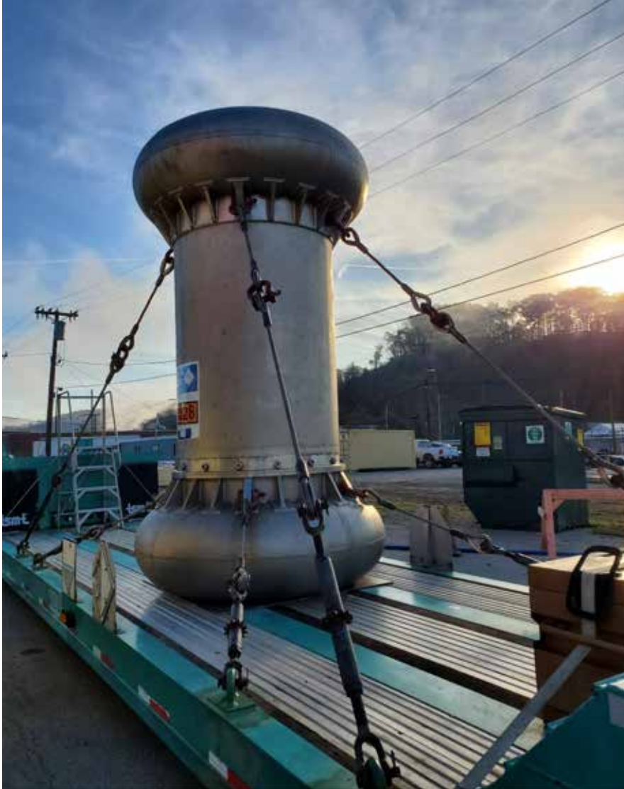
Figure 3. The GE 2000 cask containing GNF articles removed from Hatch NPS #1 delivered to ORNL hot cells
