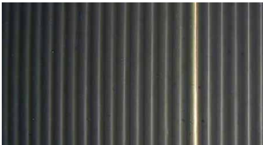
Figure 1. Cr-coated fuel rods after 1 cycle in Vogtle
