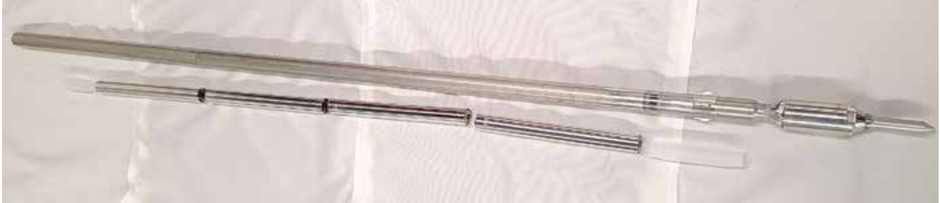
Figure 2. Parts layout for capsule assembly of tensile cladding tube specimens
