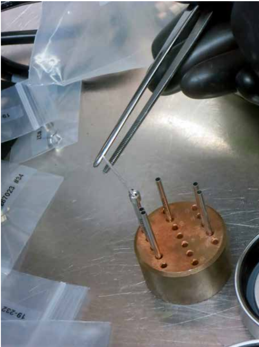
Figure 1. Technicians at the Materials & Fuels Complex (MFC) load sodium into the rodlets. All fuel fabrication and assembly work at MFC occurs within a glovebox to ensure oxidation risks are limited. After loading, the sodium is melted so that it forms a uniform bond between the fuel and cladding. The sodium is used to maintain adequate heat transfer between fuel and the cladding during early irradiation stages until the fuel is able to swell and make physical contact with the cladding.
