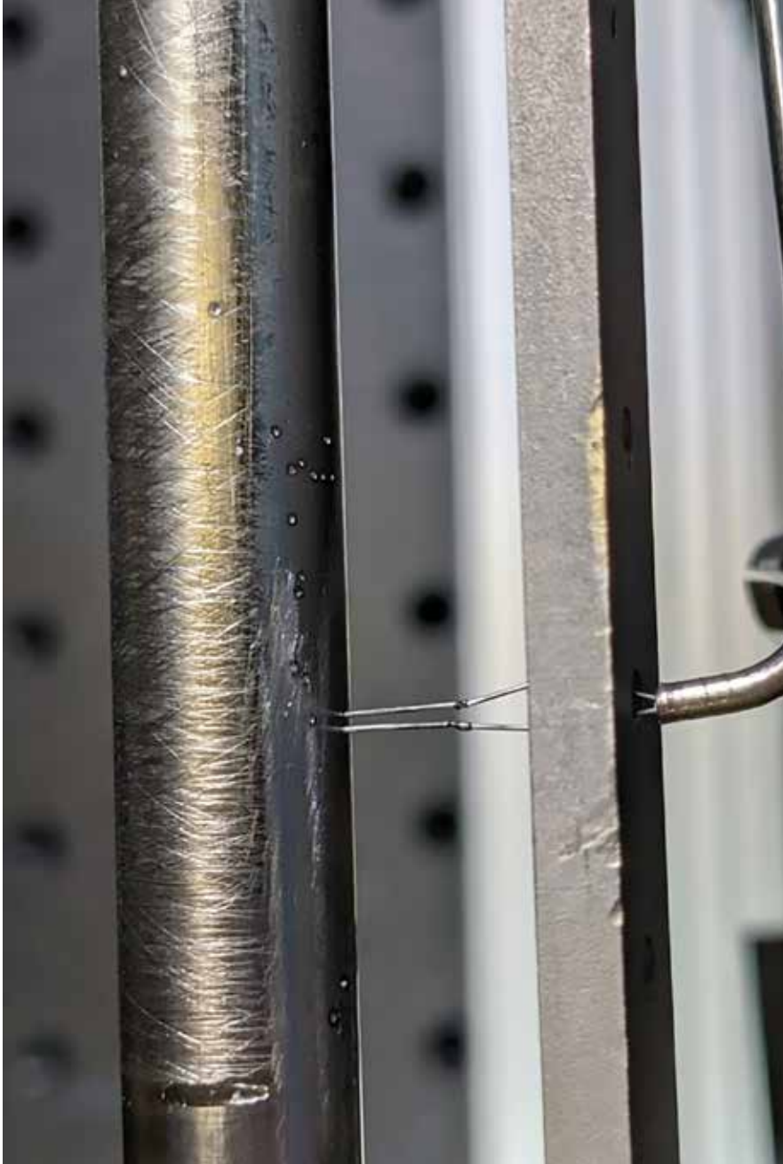
Figure 2. Cladding thermocouple weld
