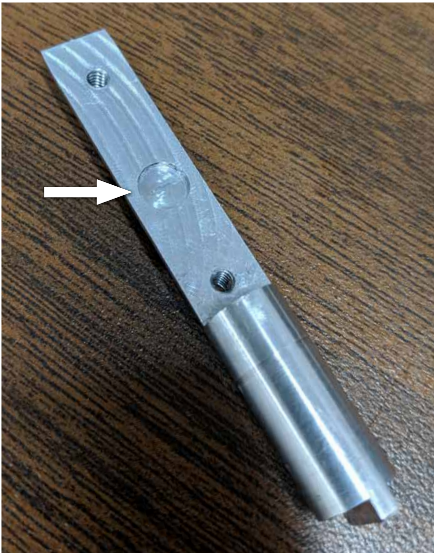
Figure 1. Opened aluminum sample holder with the cavity for the disk of irradiated U-10Zr-1Pd in the thinned section marked by an arrow (left). Sample holder closed and attached to the lid of a vanadium can that provides secondary containment of the sample (right).
