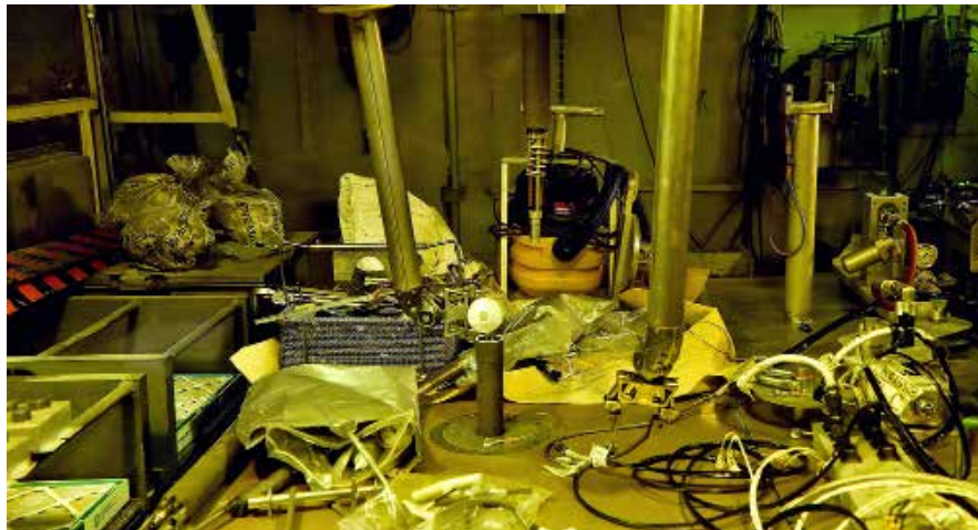
Figure 3. ATF-R experiment assembly being filled with water during assembly process at HFEF
